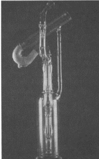
Fig. 1.1 The Lindberg-Carrel perfusion pump, 1930s, designed to keep an isolated organ supplied with enough
