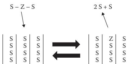
FIGURE 3.2 Presumed mechanism of competitive sorption of solute combined with dissociation of ZS_2 solvate (slope of \log k vs. \log C_{\text{mod}} plot m = 3 ). Octadecyl silica sorbent (RP-18) saturated with modifier ( S ) molecules. (Adapted from Soczewiński, E., J. Chromatogr. A , 965, 109–116, 2002.)
