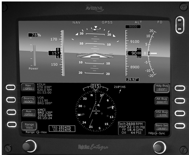
Figure 3-10. A typical primary flight display (PFD)
