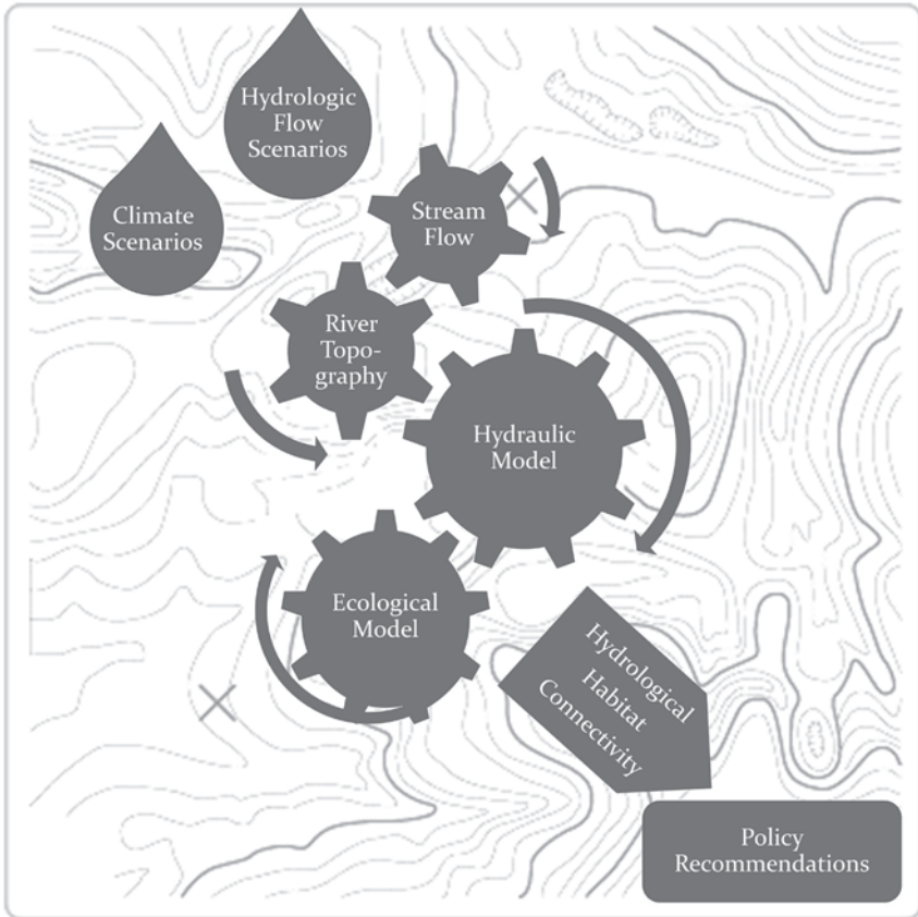
FIGURE 7.7 This integrated hydrological habitat connectivity modeling framework includes: (1) incorporation of climate change models at a fine temporal scale; (2) proposed alterations to the channel morphology at a fine spatial scale; (3) fine-scale empirical hydrology; (4) fine-scale empirical topography data; (5) spatially explicit hydraulic modeling; and (6) species and life-stage-specific ecological models; (7) to produce quantitative ecological outcomes such as changes in habitat availability; and (8) decision support for policy and management adoption. (Modified from Merenlender and Matella 2013.)
