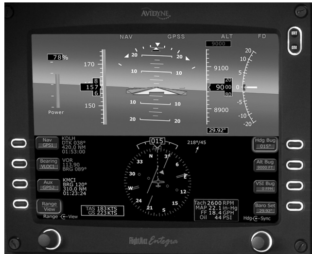
Figure 3-4. A typical primary flight display (PFD)
