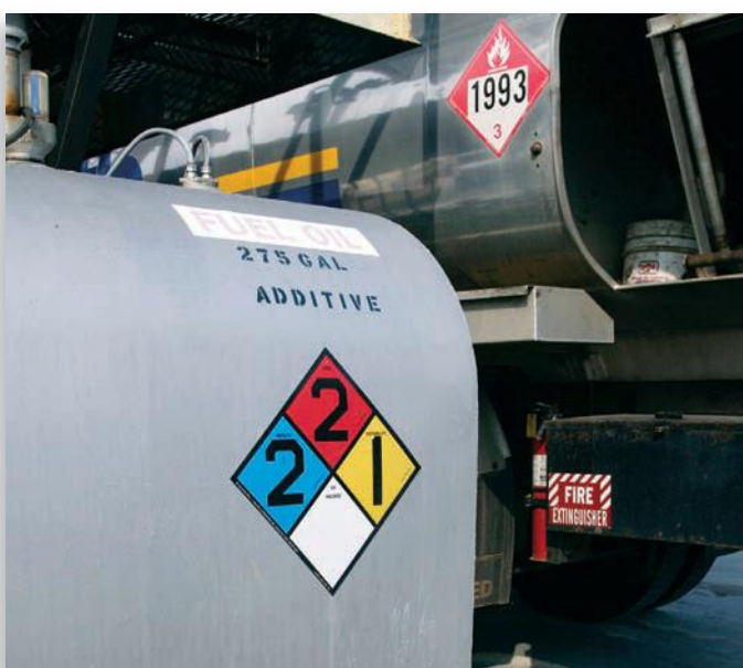
FIGURE 53-4 Placards are used to rapidly and easily identify hazardous risks.
