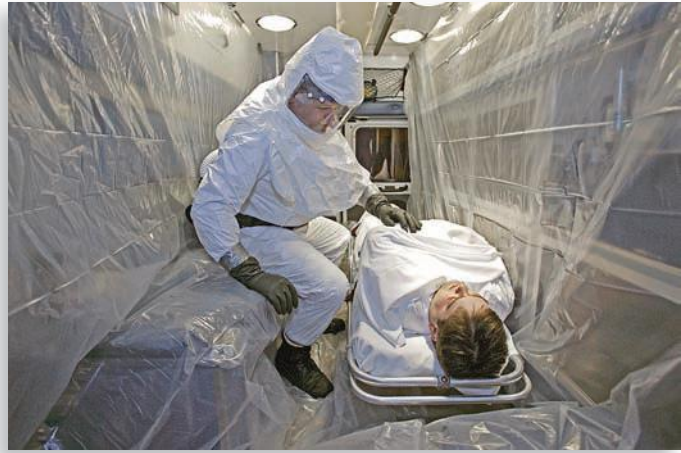
FIGURE 53-7 Enveloping involves placing a plastic barrier on the inside of the patient compartment of the ambulance so that the equipment and cabinets are protected from secondary contamination.
