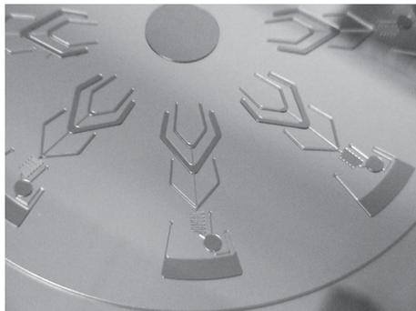
**Fig. 10.1** Image of microfluidic architectures composed of miniature microreservoirs and microchannels.
