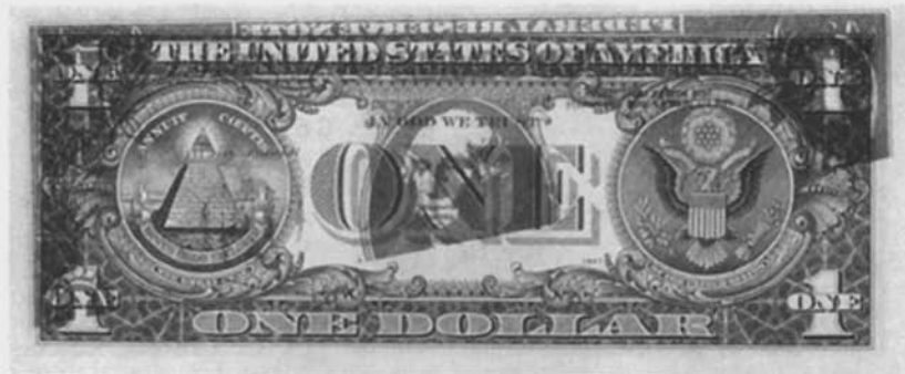
$1 FRN 1995 Fake offset generated with image reversal software. Under magnification, a faint dot matrix pattern is apparent and the color bears a brownish hue.
