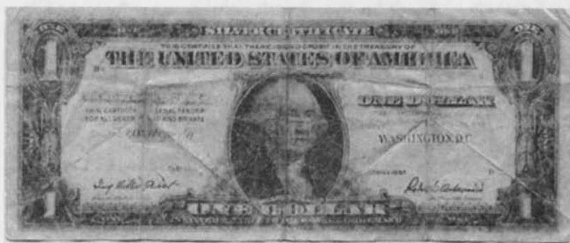
$1 SC 1957 Chemical extraction of overprint with removal of serial numbers and seal. Disturbance to remaining black ink from second printing suggests alteration.
