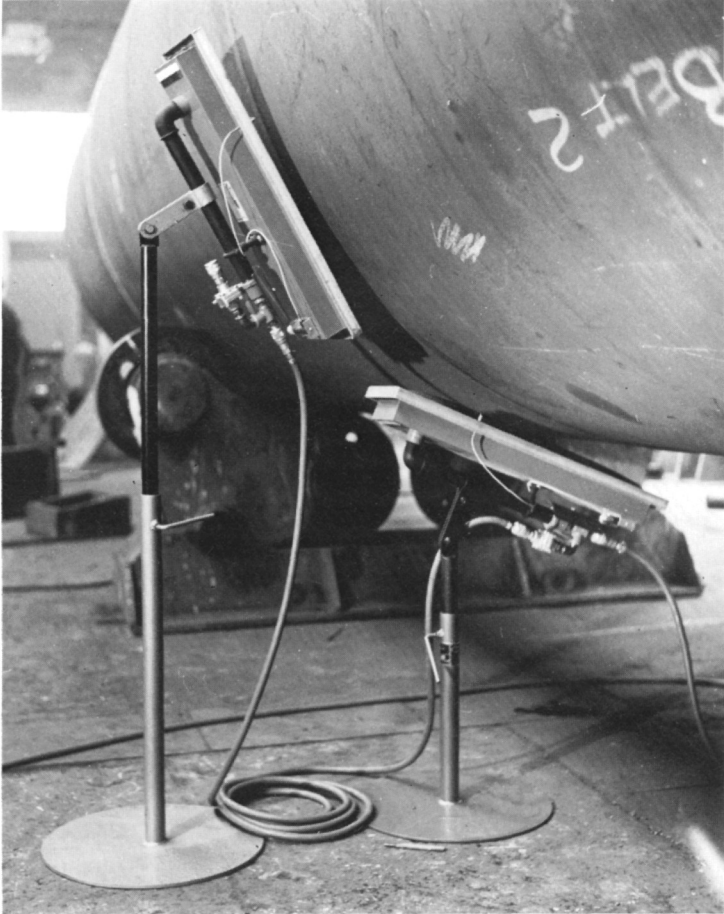
Fig. 2.40. ( b ) Surface combustion units propane or natural gas set up for pre-heating rotating seams.
