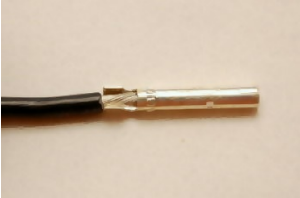
Inserting the stripped wire in the bullet connector
