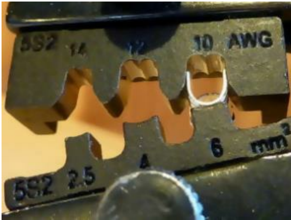
Crimping the wire inside the connector
