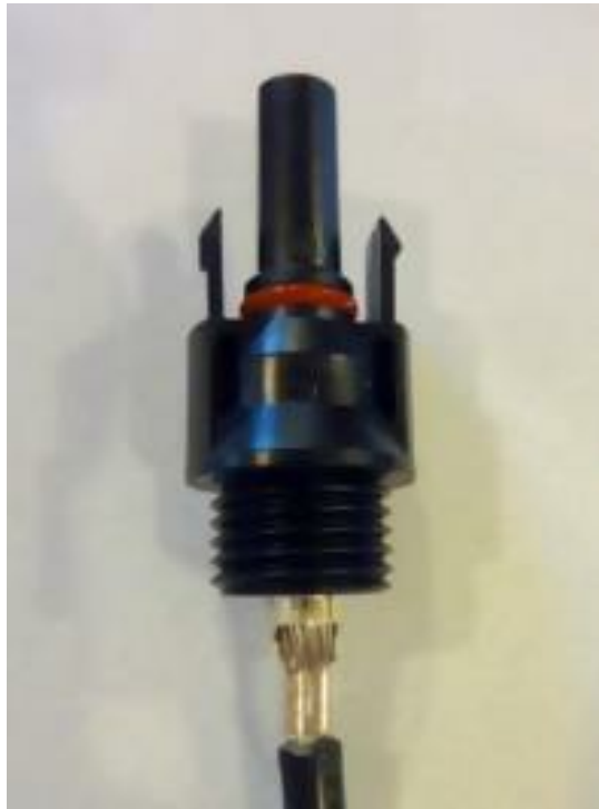
Inserting the crimped connector in the MC4 housing Source: Marine How-To
