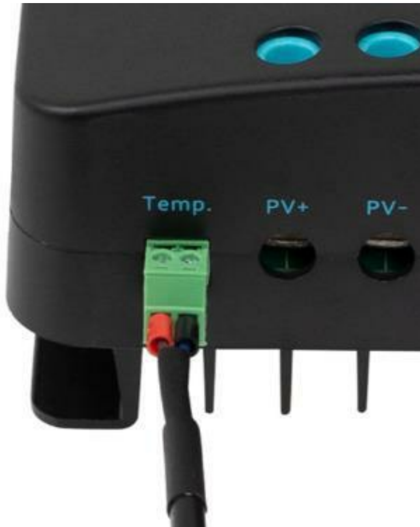
Temperature compensation on the Renogy charge controller
