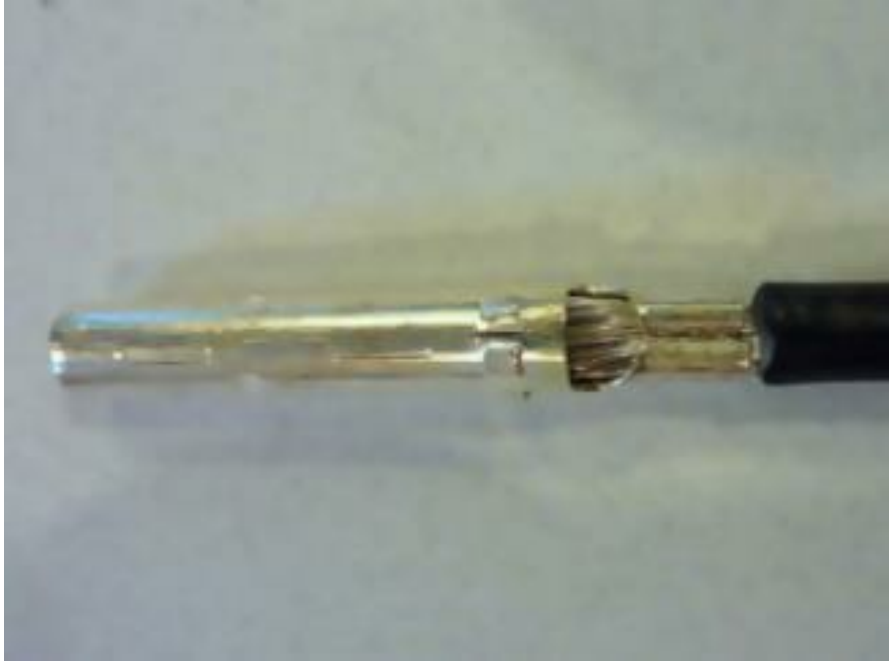
Crimped wire inside the connector
