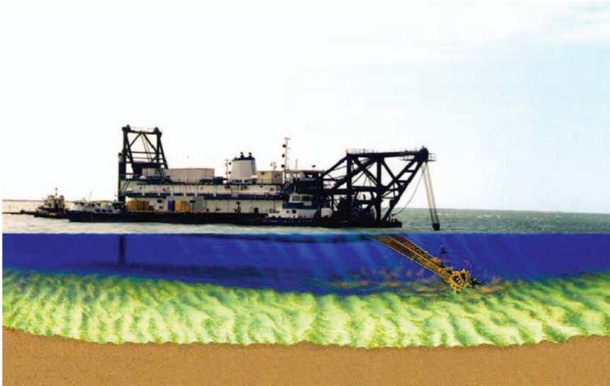
Figure 9-3. Hydraulic cutterhead dredge.
