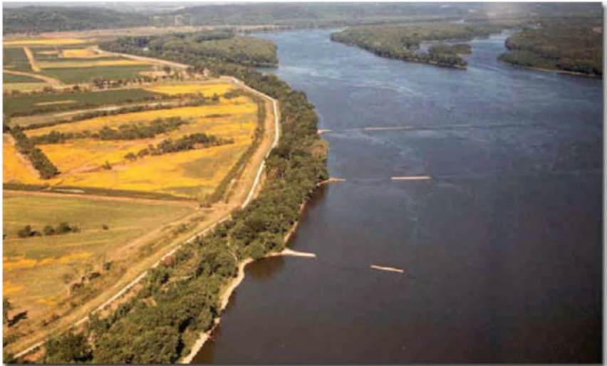
Figure 10-4. Stone spur dikes with notches.
