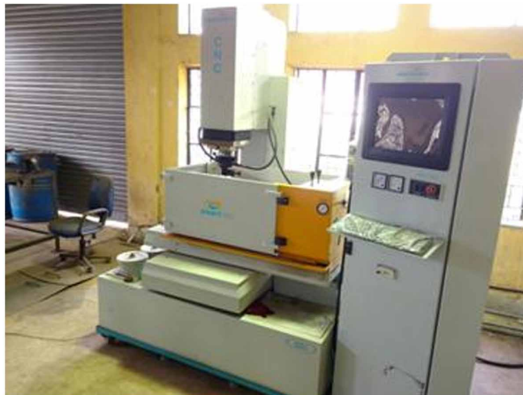
Figure 1. Electric discharge machine setup
