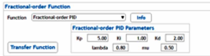
Figure 4. Parameters window for the fractional-order PID controller
