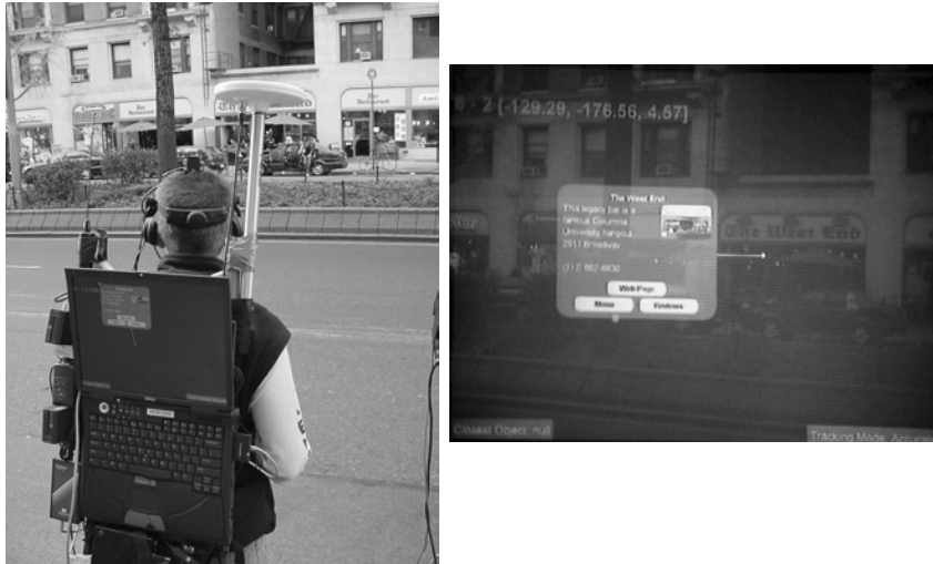
Figure 21. Outdoor augmented reality environment: (a) Backpack system, (b) information about the restaurant is seen in the user's view through a head-worn display
