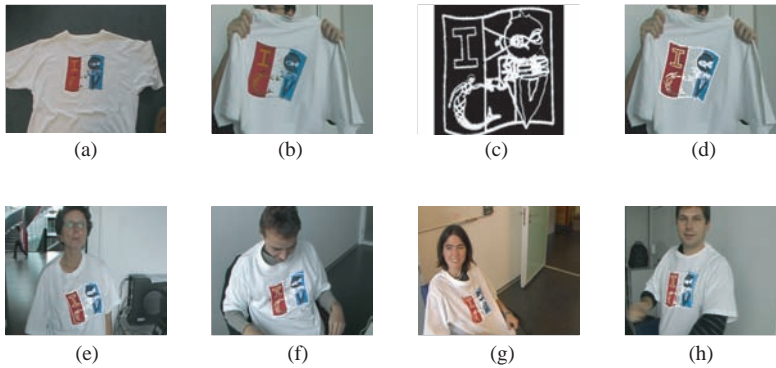
Figure 6. Real-time detection of a deformable object. Given a model image (a), the algorithm computes a function mapping the model to an input image (b). To illustrate this mapping, the contours of the model (c) are extracted using a simple gradient operator and used as a validation texture which is overlaid on the input image using the recovered transformation (d). Additional results are obtained in different conditions (e)-(h). Note that in all cases, the white outlines project almost exactly at the right place, thus indicating a correct registration and shape estimation. The registration process, including image acquisition, takes about 80 ms and does not require any initialization or a priori pose information. (Reproduced from Pilet et al., 2005a, © 2005 IEEE, used with permission)
