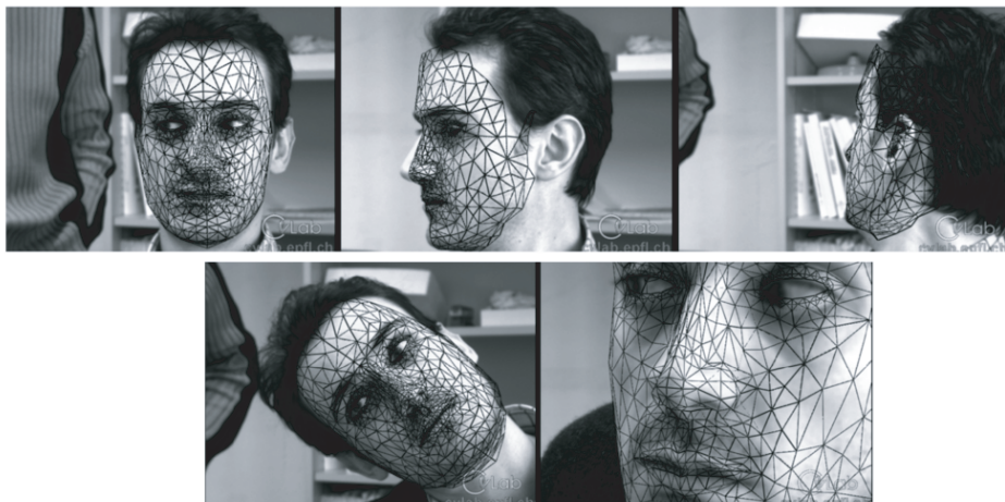
Figure 3. Face tracking using interest points, and one reference image shown (top left) (Reproduced from Vacchetti et al., 2004b, © 2004 IEEE, used with permission)
