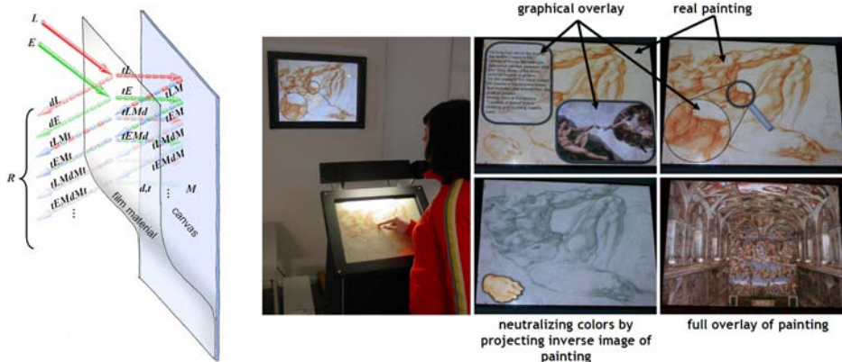
Figure 4. Interaction of projected light and environment light with the screen canvas and the transparent projection film—sequence diagram (right); examples of interactive projections onto real painting (right) (Images reprinted from Bimber et al., 2005a, © IEEE)
