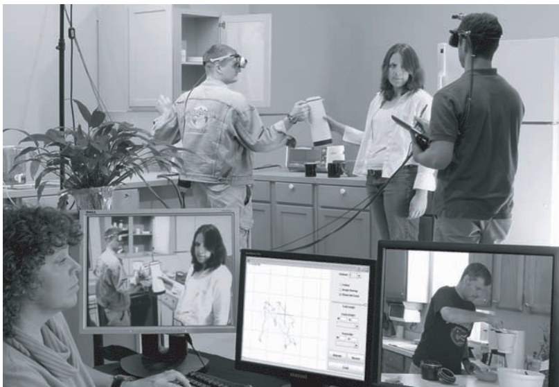
Figure 11. Human experience modeler capturing, simulating, and analyzing human performance with cognitive rehabilitation for retraining of daily activities for traumatic brain injury patients (©2006 Media Convergence Laboratory/UCF, used with permission)
