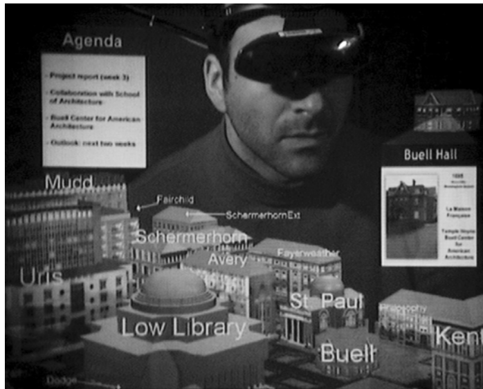
Figure 2. View management in an augmented reality meeting scenario (Imaged through a tracked, optical see-through, head-worn display)
