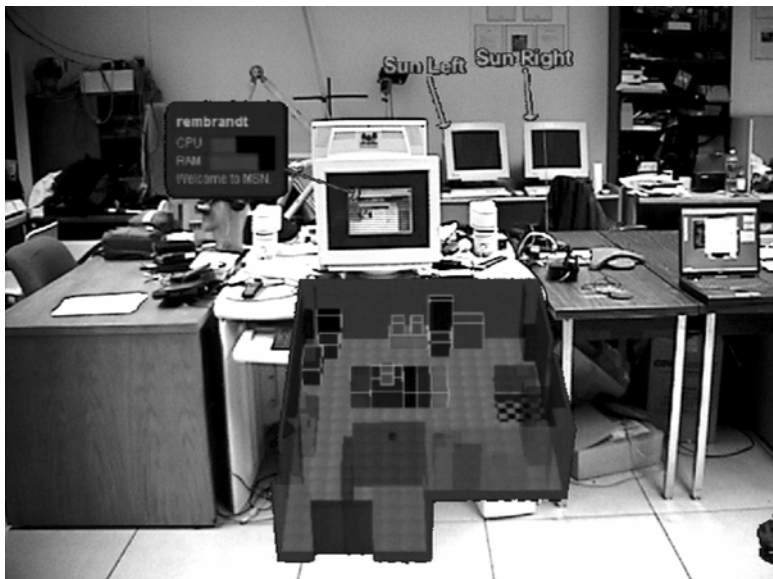
Figure 22. Augmented reality user interface that incorporates a world-in-miniature to give the user a better understanding of their environment
