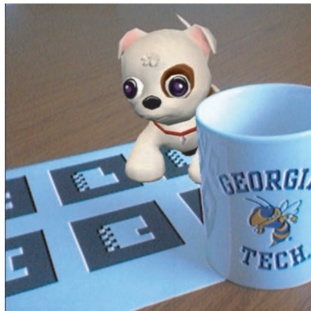
Figure 5. The physical object (the cup) occludes the virtual object (the dog)
