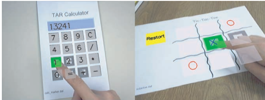
Figure 9. Occlusion-based Interaction with calculator and tic-tac-toe game
