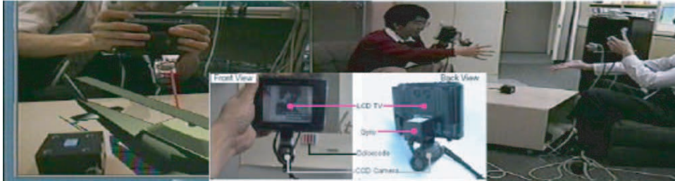
Figure 1. The pioneering system, Transvision, which consisted of a small LCD display and camera and allowed collaborative hand-held augmented reality interaction (Rekimoto, 1996) (Image courtesy of Jun Rekimoto, Sony CSL)
