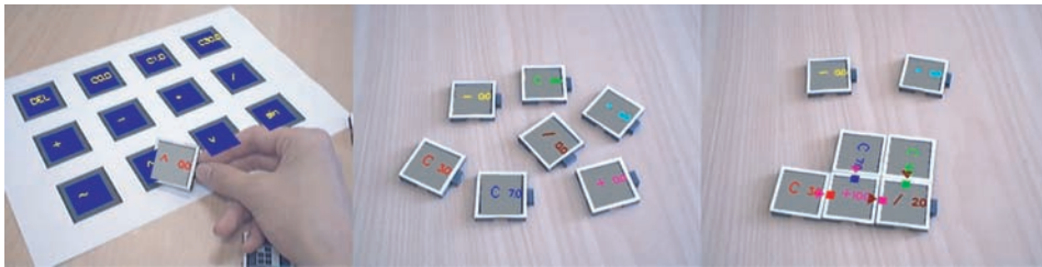
Figure 7. A Tangible AR puzzle calculator: A data flow graph for calculating a mathematical expression is made by connecting puzzle pieces with mathematical entities
