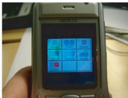
Figure 5. The semi-transparent menu for selecting transformation mode
