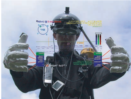
Figure 7. Each finger maps to a displayed menu option, the user selects one by pressing the appropriate finger against the thumb
