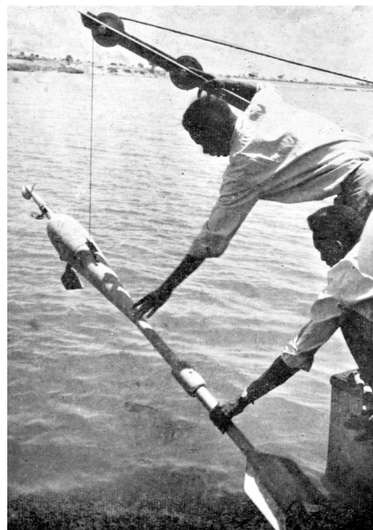
Fig. 4.10 Propeller-type Current Meter—Neyrtec Type with Sounding Weight
