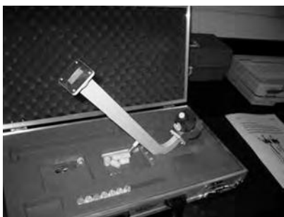
Figure 11.10 An X-band resonant cavity, with waveguide attached. Note the dimensions of ~3 cm (Courtesy: Alan Wilder, UC Davis ChemWiki)
