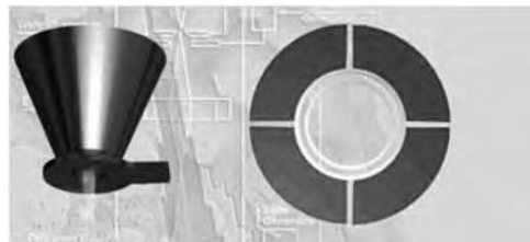
Figure 13.15 Shows Typical 4 quadrant solid state BSE detector (Courtesy: M/s Oxford Instruments Microanalysis Group: The Oxford Guide to X-Ray Microanalysis )
