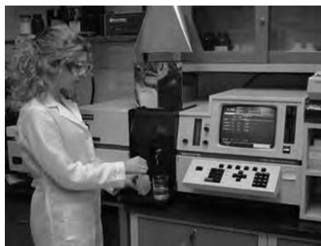
Figure 5.14 Atomic Absorption Spectrophotometer Varian Spectra 10/20 for analysis of metals in the ppm range with flame, and ppb range with graphite furnace (Courtesy: M/s Varian)
