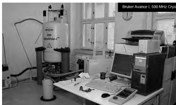
Figure 10.9 Typical 500 MHz FT-NMR spectrometer (Courtesy: M/s Bruker)
