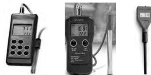
Figure 23.7 Portable pH metre (Courtesy: M/s Hanna Instruments, www.hannainst.com )
