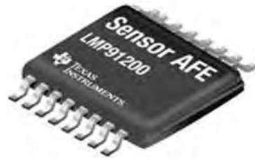
Figure 23.13 LMP91200 pH Sensor integrated circuit (Courtesy: M/s Texas Instruments)
