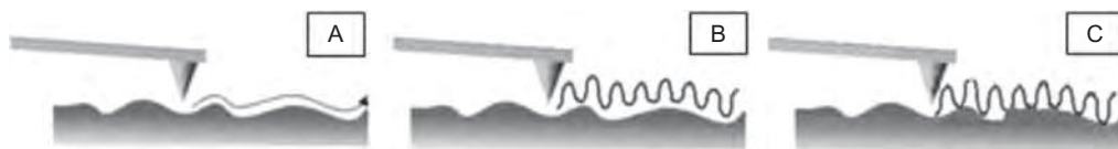
Figure 14.10 Different modes of operation of STM (a) Contact mode; (b) Non-contact mode; and (c) Tapping mode (Courtesy: M/s Pacific Nanotechnology, 2006)
