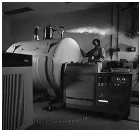
Figure 9.21 A typical FT-ICR mass spectrometer (Courtesy: M/s Thermo Fisher)
