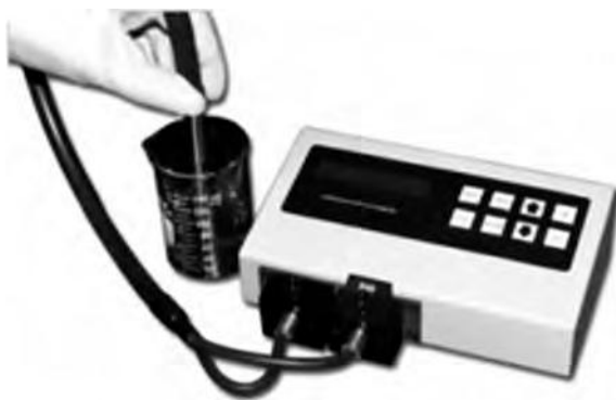
Figure 2.38 Photograph of a probe-type photometer. (Courtesy : M/s Metrohm USA)
