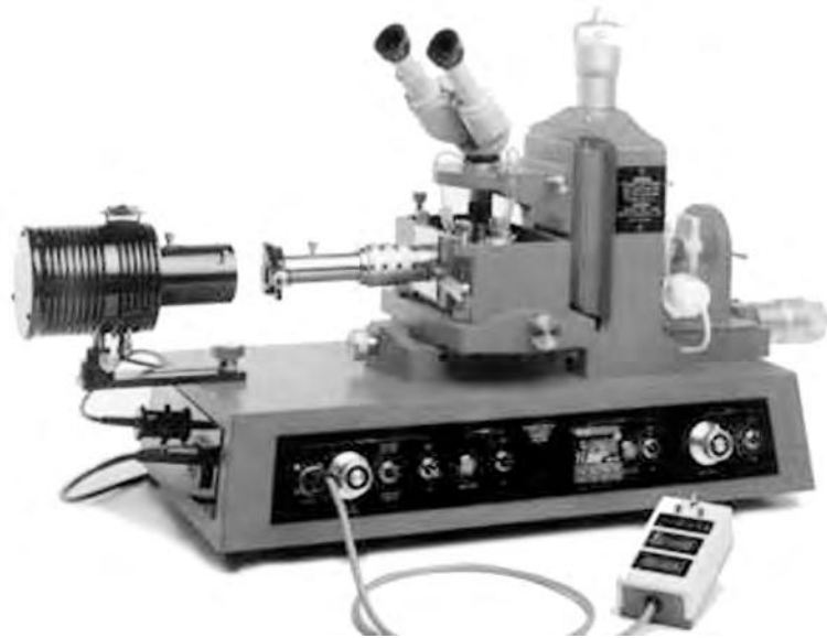
Figure 21.9 Micro-electrophoretic apparatus (Courtesy: M/s Rank Brothers Ltd. UK)
