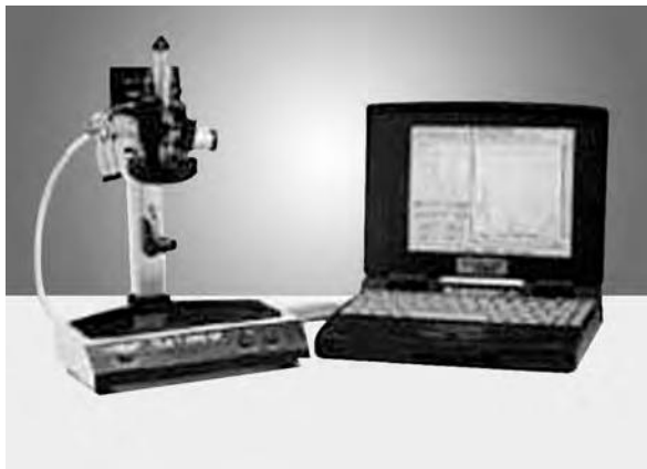
Figure 22.20 Polarography-voltammetry system with PC support (Courtesy: M/s Topac, USA)
