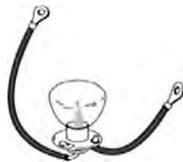
Figure 2.12a A tungsten lamp of the type used in absorption instruments (Courtesy: M/s Thomson Higher Education)
