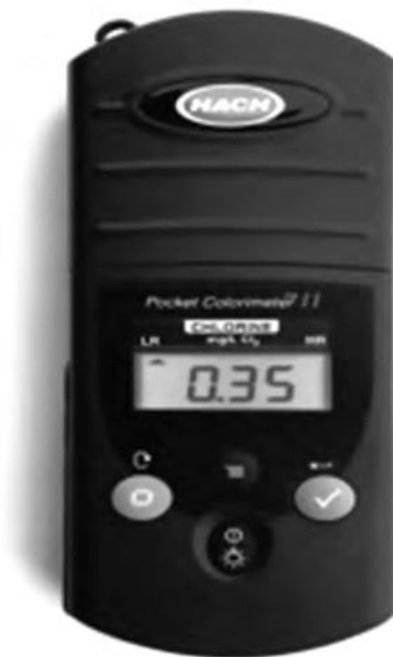
Figure 2.41 Photograph of a simple LED-based colorimeter. (Courtesy : M/s HACH Lange, UK )
