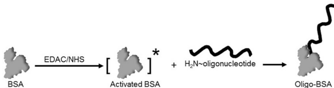
Fig. 12 Coupling of capture oligonucleotide to BSA. Bovine serum albumin carboxyl groups are converted to NHS esters to form activated BSA. The BSA-NHS ester reacts with amine-terminated oligonucleotides, resulting in the formation of oligo-modified BSA
