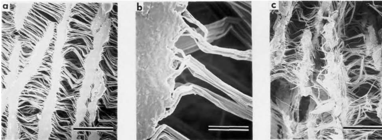
Figure 5. Low voltage scanning electron microscopy of modified ePTFE. Images were collected at the superficial luminal surfaces at low magnification (a, d, g; 1000\times , bar = 30\ \mu\text{m} ) and at high magnification (b, e, h; 20\,000\times , bar = 1.5\ \mu\text{m} ); and approx. mid-way across the graft wall in cross-sections (c, f, i; 1000\times , bar = 30\ \mu\text{m} ). Images at high magnifications were obtained at the center of the lower magnification regions. The outer superficial surface appeared very similar to the luminal superficial surface and is not shown here. (a, b, c) Control unmodified ePTFE; (d, e, f) ePTFE thermochemically reduced at a reaction temperature of 105^\circ\text{C} for 1 day; and (g, h, i) ePTFE photograft polymerized with comonomers of PEG-Ac 200 and PEG-Ac 8000 by UV irradiation for 1.5 h on the thermochemically reduced substrate.
