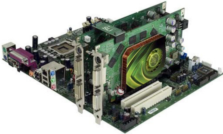
Figure 4.19. The SLI by Nvidia. For a color version of this figure, see www.iste.co.uk/darche/microprocessor2.zip
