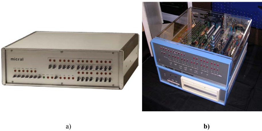
Figure 1.24. The first microcomputers: the Micral N from R2E and the ALTAIR 8800 from the American company MITS (source: unknown). For a color version of this figure, see www.iste.co.uk/darche/microprocessor1.zip
