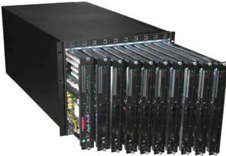
Figure 1.28. A blade server. For a color version of this figure, see www.iste.co.uk/darche/microprocessor1.zip
