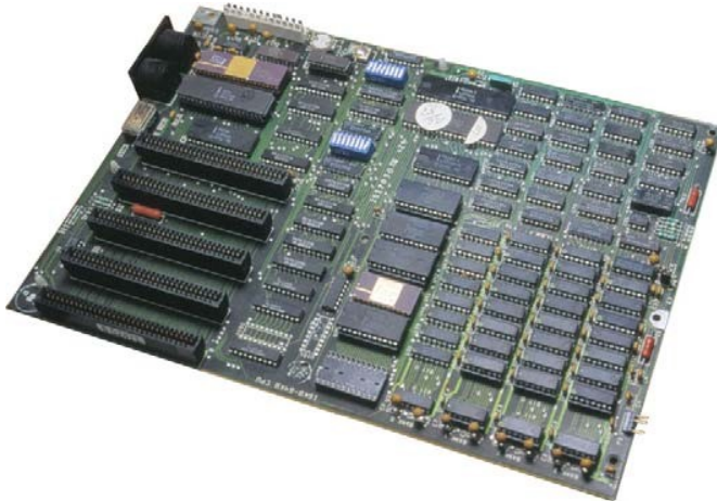
Figure 1.16. PC motherboard (5150) from IBM (1981). For a color version of this figure, see www.iste.co.uk/darche/microprocessor1.zip
