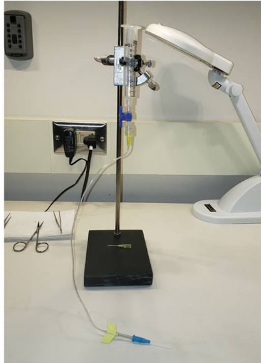
Fig. 4 Syringe and catheter setup to prepare formalin-inflated lungs. A 10-mL syringe is held in place by a clamp such that the 10-mL mark on the syringe is 20 cm above the benchtop. The blue stopcock controls the flow of formalin. The catheter is placed into the trachea during instillation of formalin
