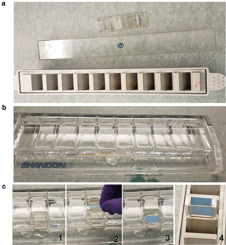
Fig. 2 The use of Shandon™ Sequenza™ Staining Rack and coverplates allows for controlled flow of 200 \mu L of fluid over slides and for several slides to be processed at the same time. (a) Shandon™ Sequenza™ Staining Rack, lid, and coverplate. There is room for ten slides per rack. (b) Slide preparation rack filled with distilled water. (c) Instructions of how to load slides onto coverplate: (1) A container is filled with water; (2) Coverplate is submerged under water; (3) A slide is lowered onto the coverplate face-down, creating a small water filled void between the slide and coverplate; (4) Hold in place and then slide into the rack firmly
