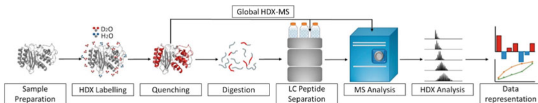
Fig. 2 A general experimental workflow for continuous labeling HDX-MS. (Reprinted from ref. 3 with permission from Elsevier)
