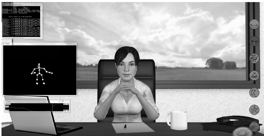
Figure 29.4 The virtual job interview training environment. On the right side there are feedback signal lights providing feedback for nonverbal and paraverbal behavior (smiling, eye contact, body posture, arm position, nodding, voice loudness, vocal energy). On the left side there is the recognized skeleton of the participant and below there is a continuous smile analysis.
