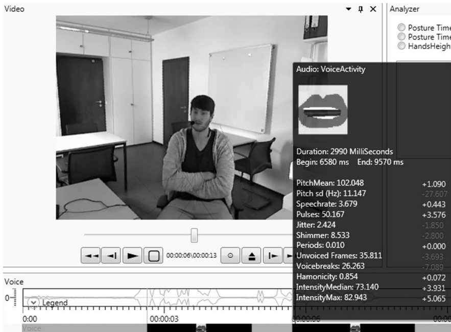
Figure 29.1 Output example of a voice analysis with PRAAT within the graphical user interface NovA ( The [Non]Verbal Annotator , Baur et al., 2013). In the middle there is the voice activity detection. For instance, it indicates that the person speaks with a voice intensity of 73.140 dB (median) during this specific voice activity (i.e., the person talked for a duration of 2990 milliseconds during this voice activity).
