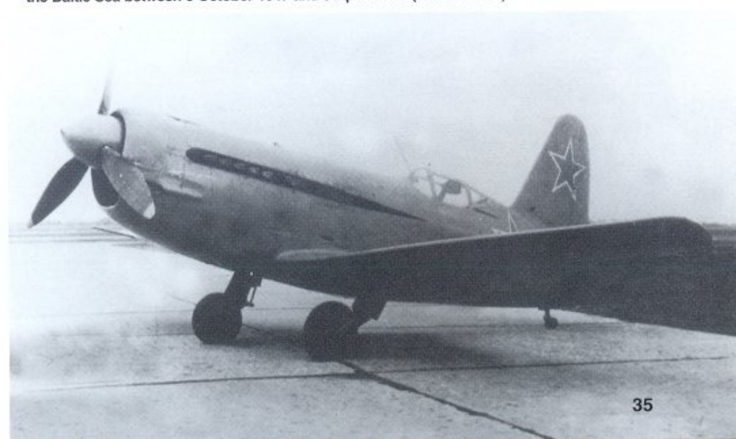
▼ Only ten MiG-13s were built, all at State Aircraft Factory 381 at Yaroslavl. In contrast to the N-2, the MiG-13 had a taller tail and an antenna mast raked forward and to starboard. This is the second production MiG-13 (serial number 3810102), which was evaluated by the Aviatsiya Voyenno Morskogo Flota (Soviet Naval Aviation) at Skulte aerodrome near Riga on the Baltic Sea between 9 October 1947 and 3 April 1948. (Robert Bock)
