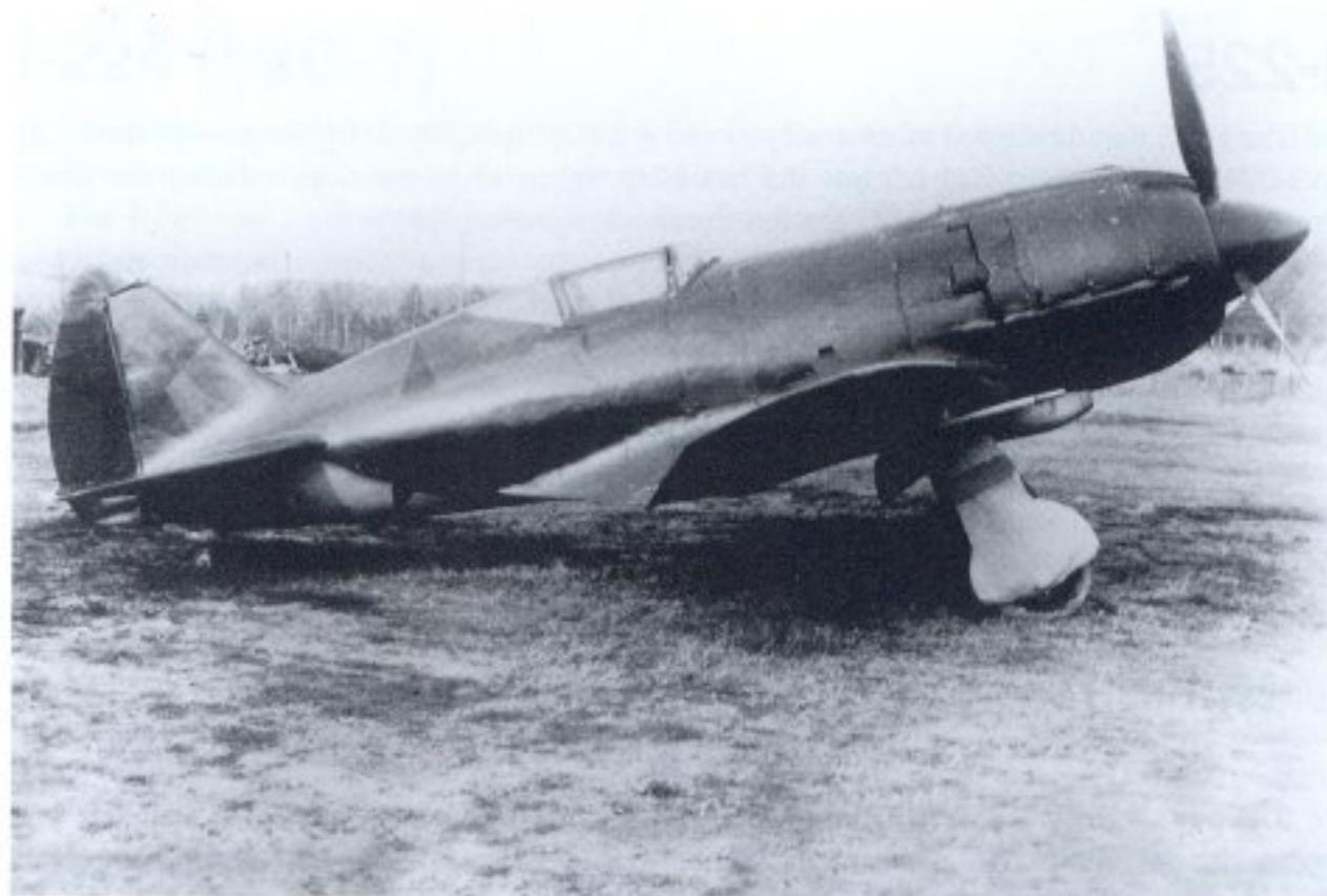
▲ The I-210 was the first attempt of the MiG Design Bureau to mate the M-82A radial engine with the fuselage of the MiG-3. The cockpit canopy was enlarged on the I-210 and deepened to improve rear visibility. (G.F. Petrov)
