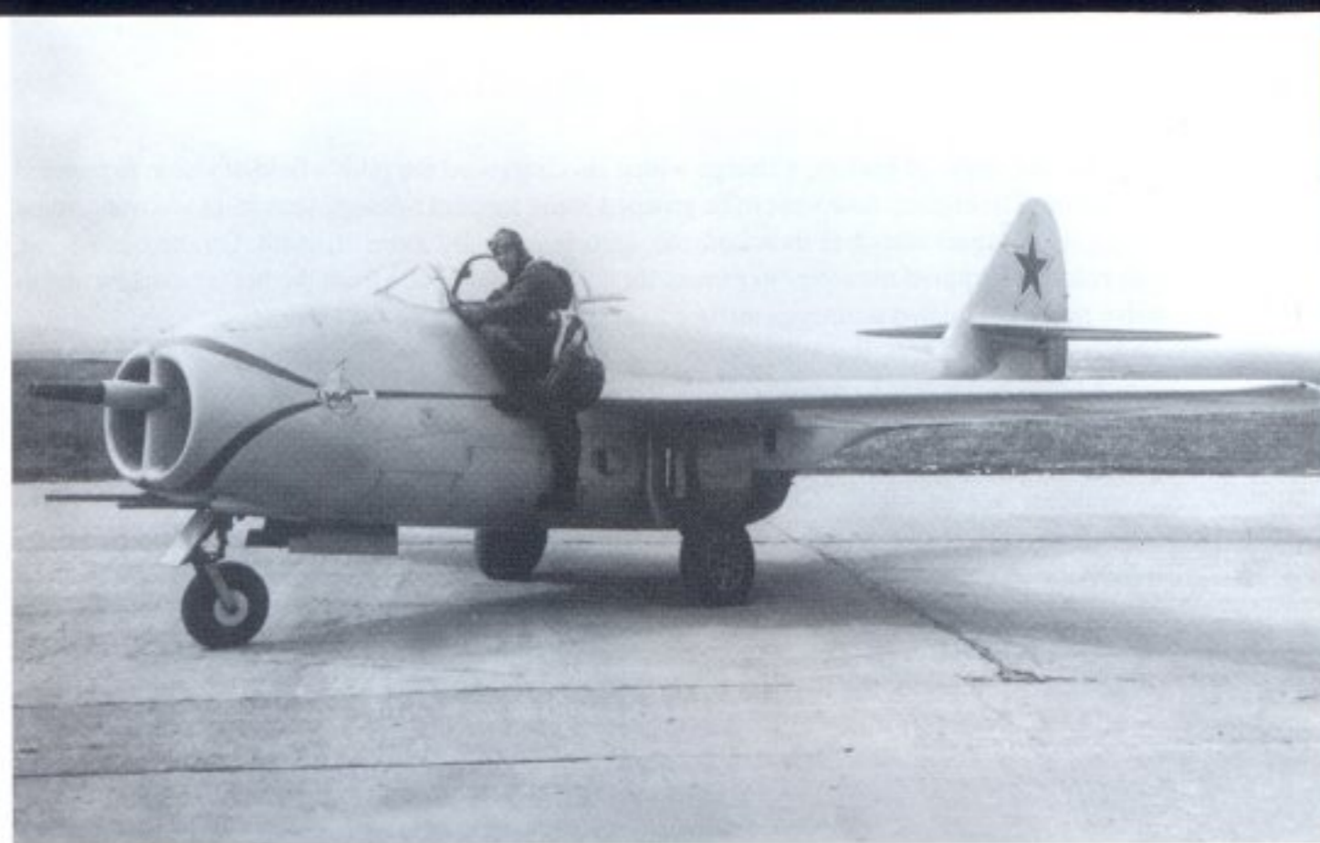
▲ The MiG-9 was the great-grandmother of all jet-powered MiG fighters, and the prototype MiG-9/I-300 (F-1) was the first Soviet jet to fly. This historic event took place 24 April 1946, when Aleksey Nikolayevich Grinchik took off from Kratovo (Ramenskoye) with the F-1 prototype. The I-300 was powered by two German BMW 003A-1 engines that had been built in the Bavarian Motor Works plant at Basdorf-Zühlsdorf. (G.F. Petrov)
