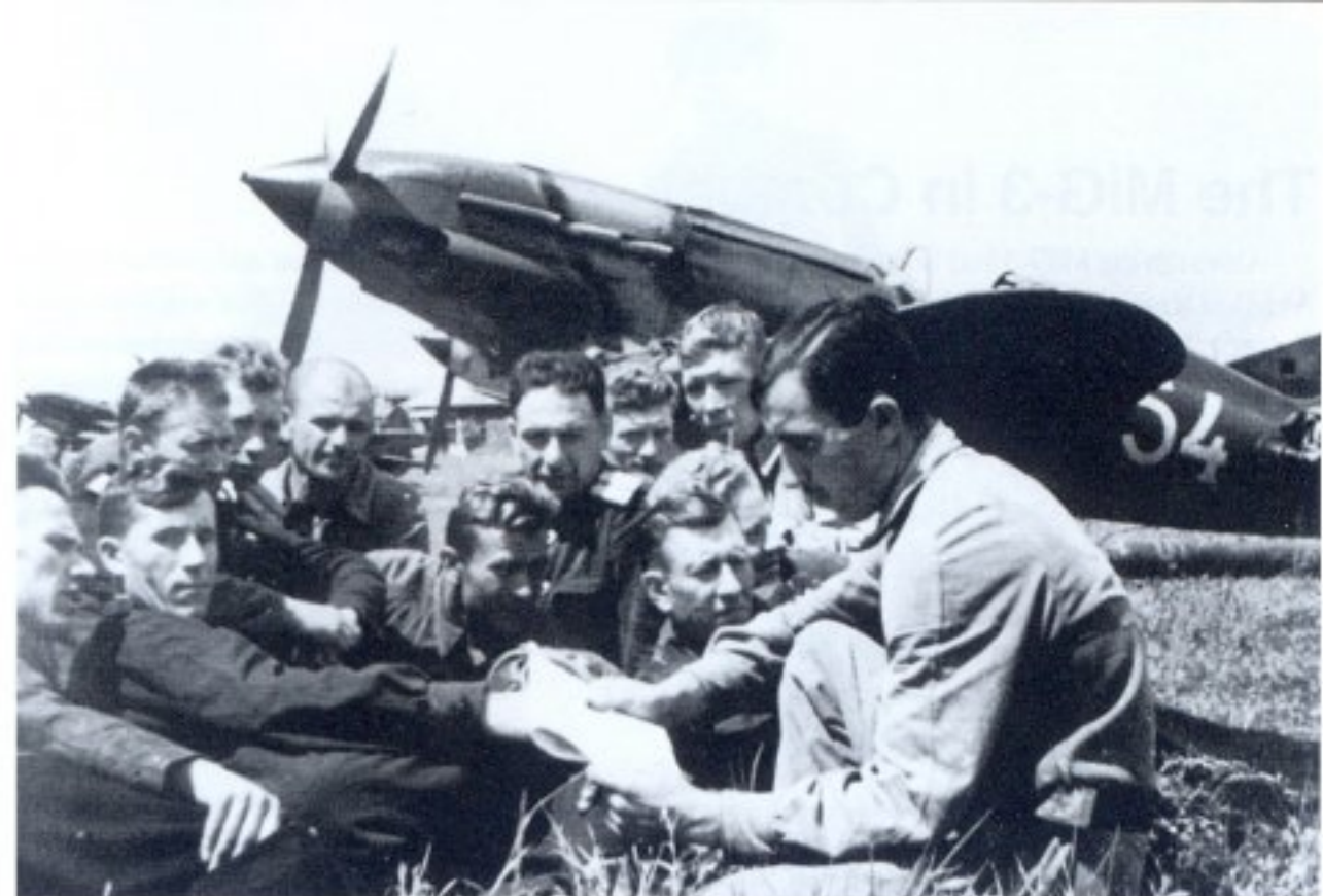
▲ 'White 54' of the 34. IAP is unusual in having a Hucks-type starter lug fitted on the propeller hub. Only a very few MiG-3s were so equipped. The MiG-3 carries a camouflage of 'All' Green and 'All' Dark Green on the upper surfaces and 'All' Blue on the lower surfaces. The Black stripes applied in the 'All' Dark Green areas are unusual. The lack of a national insignia on the rear fuselage is not standard for 1943; in late June 1941 a directive was issued that all MiG-3s were to have a red star painted on the rear fuselage as well as the tail. (Robert Bock)
