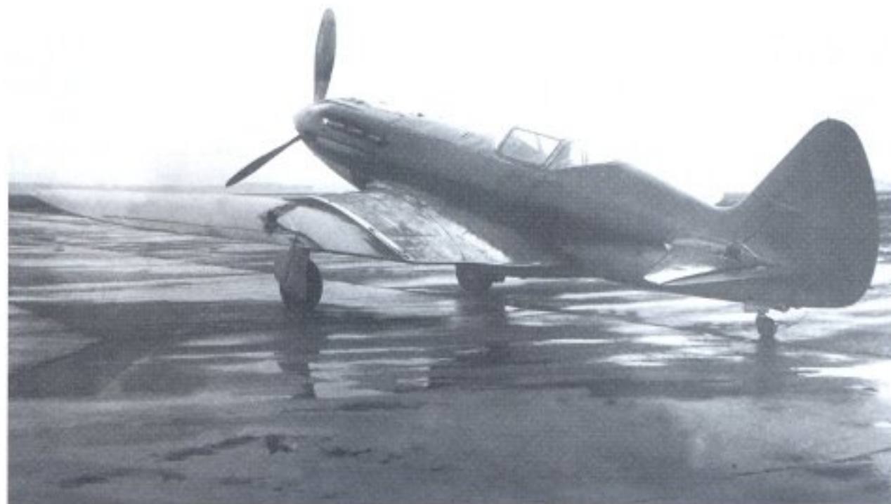
▲ An early production MiG-3 during flight evaluation with the Nauchno-Ispitatel'niy Institut Voenno-Vozdushikh Sil (Scientific Research Institute of the Soviet Air Force) at Chalovskaya Air Base. The first production MiG-3s lacked the four blisters on the upper engine cowling which were introduced on subsequent production batches to allow proper function of the two 7.62 mm ShKAS machine guns. The MiG-3 is painted in Factory Green with 'All' Blue undersurfaces. No national markings have been applied to this particular aircraft. (G. F. Petrov)
