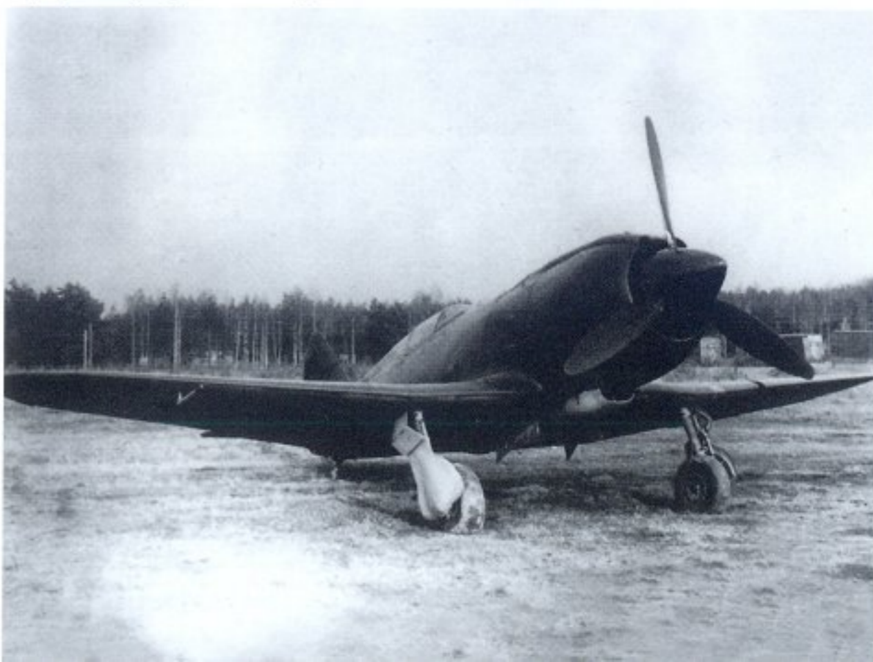
▼ The first I-210. The M-82A engine had a takeoff rating of 1,676 hp and turned an AV-5L-156 propeller. (Sergei Kuznetsov)
