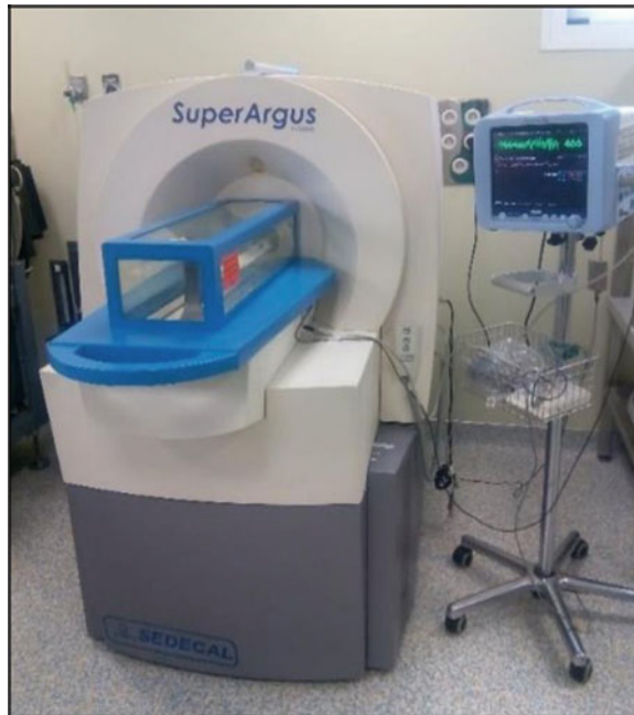
Fig. 3 Preclinical PET/CT scanner (Super Argus, SEDECAL, Madrid, Spain) at the Medical Imaging Laboratory (LIM) at the Gregorio Marañón Health Research Institute (Spain). The scanner is connected to an animal monitoring system (VisionPET, RGB, Madrid, Spain) that measures multiple physiological parameters (temperature, electrocardiogram and respiration, and optionally, oxygen saturation, blood pressure, and exhaled CO 2 ). Picture is courtesy of the head of LIM, Dr. Manuel Desco
