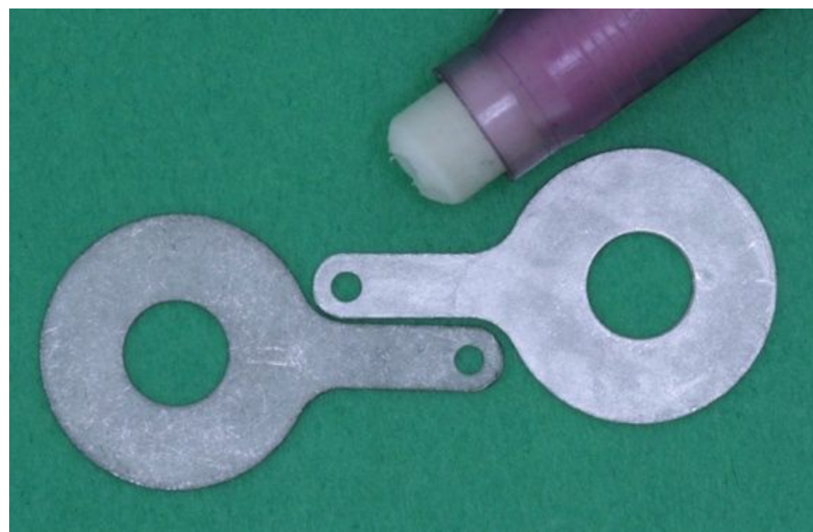
Figure 4-8 Using an abrasive stick (white eraser) to remove heavy oxidation. You can see the improvement in the part to the right. is applied to the largest thermal
