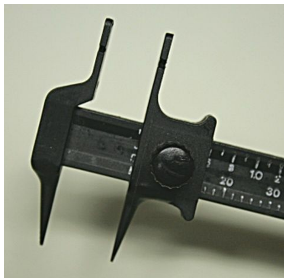
Figure 6-28 Subtract two minor divisions from the reading noted in Figure 6-27 .
