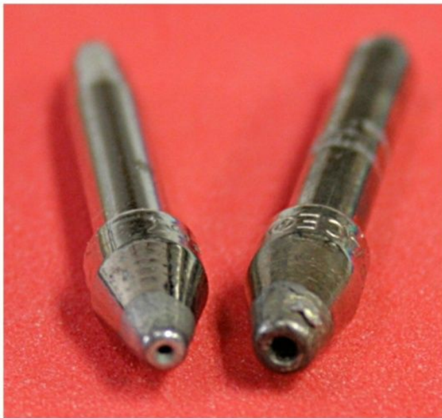
Figure 6-49 Just two tip sizes available for a constant vacuum extraction tool.
