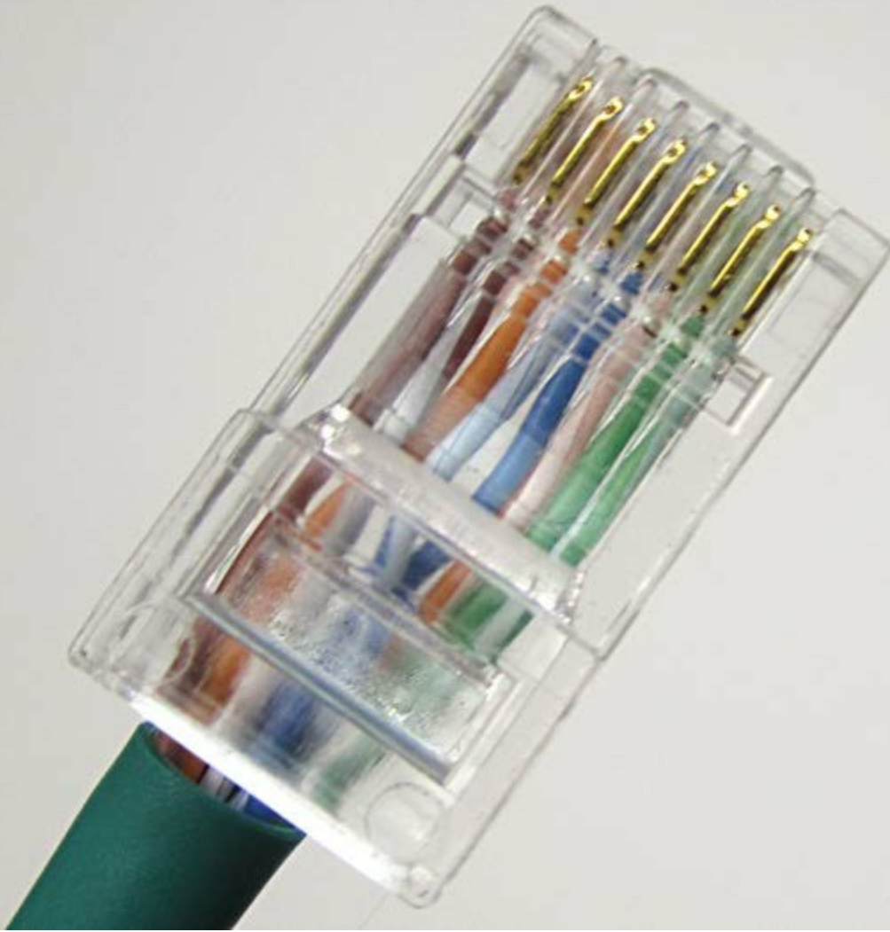
Figure 2-42 A poor crimp, the sleeve is not under the locking flange.
