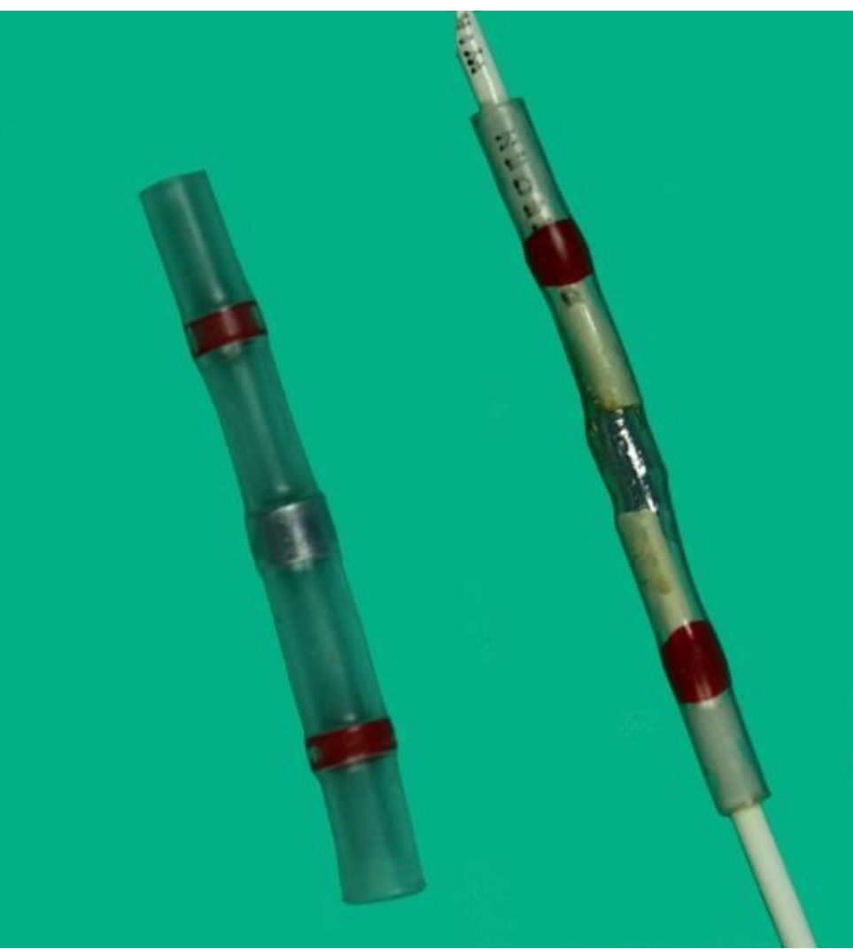
Figure 2-17 A solder splicing sleeve before and after use.
