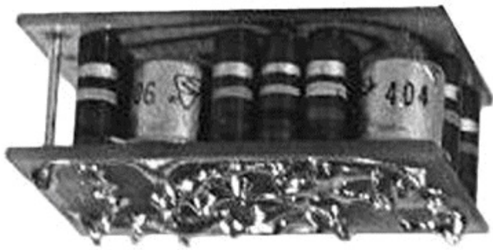
Figure 5-2 A board using cordwood construction.
