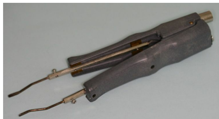
Figure 4-24 Figure 4-25 One of the many resistive tweezers available to the technician. place.
