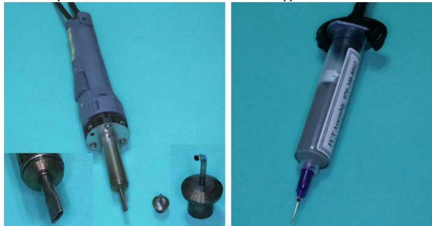
Figure 7-20 A thermal hand piece and two of many available tips.
