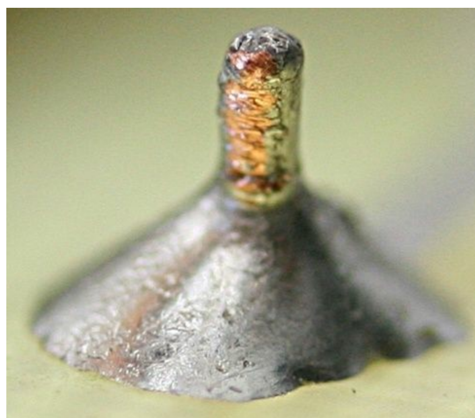
Figure 6-22 Damage to the base metal. This component will have to be replaced.
