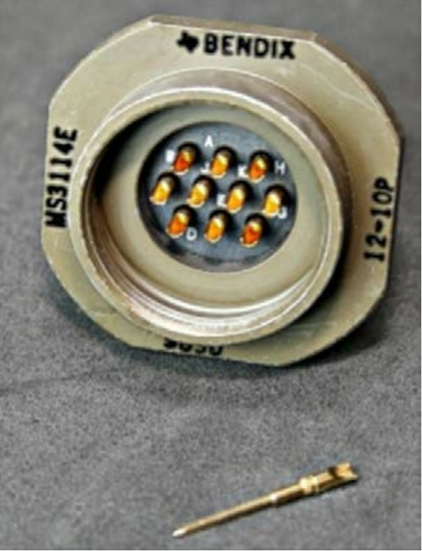
Figure 4-20 This shell has 10 pins; some can have almost a hundred.
