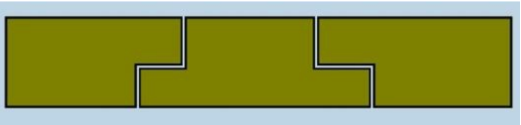
Figure 8-42 With patience, the part can be cut to fit the repair area precisely. Epoxy can be used to finalize the repair.
