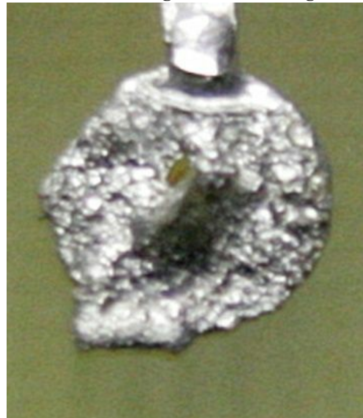
Figure 6-19 An extreme example of a cold solder joint.
