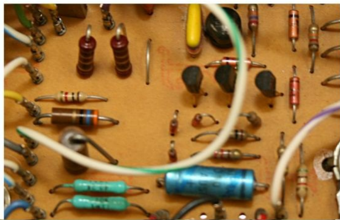
Figure 5-3 Figure 5-4 FR-1 Board FR-2 Board made of Bakelite
