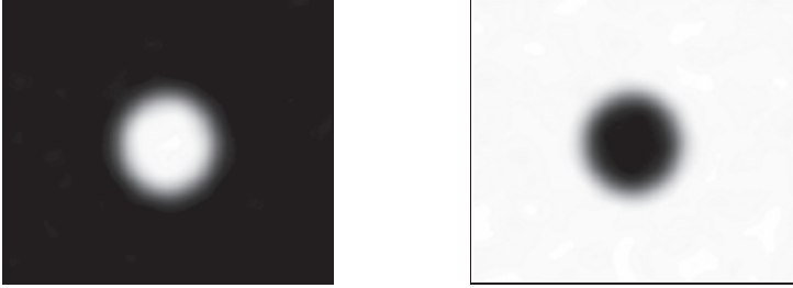
Figure 18.6 Illustration of exemplar classifier output for a hot insert, where the insert contains a greater concentration of the radio-pharmaceutical to simulate increased biological uptake often associated with pathological conditions such as a tumor. The left image corresponds to the insert mixing value ( \xi = \xi_1 ) and the right corresponds to the complementary mixing component ( (1 - \xi) = \xi_2 ). Brightness is proportional to the magnitude of the mixing present for hot insert (left) and background (right). © 2007 IEEE. Reprinted, with permission, from K. Wells et al., Quantifying the Partial Volume Effect in PET Using Benford's Law , IEEE TNS 54 (5:1), 2007 pp. 1616–1625.
