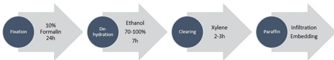
Fig. 1 Scheme of the standard procedure for FFPE samples preparation
