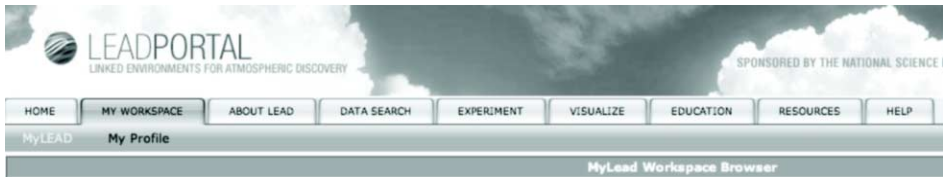
Figure 2. The collection of portlets in the LEAD portal are organized by tabs. Each major tab leads to a second level of portlets. In this case the user has selected "My Workspace" and then the user metadata catalog browser "MyLEAD".
