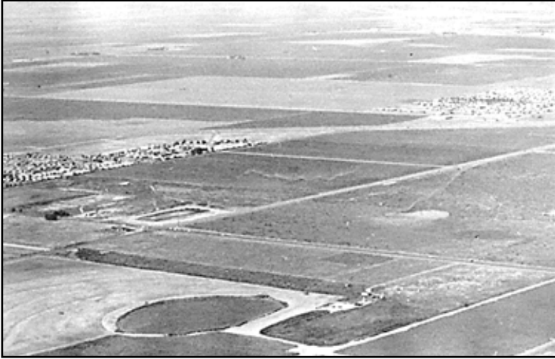
Figure 2-4. Typical terrain representative of Exposure C.
