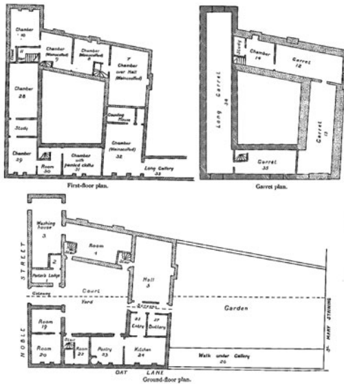
Fig. 3. Plans of Bacon House. Scale 20 ft. to 1 in. The shading shows the division of the several floors in 1625.
