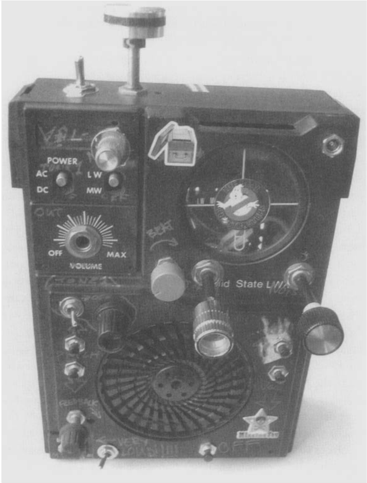
Ghostbox : circuit-bent toy by Tim Drage. Copyright 2003 Tim Drage, www.cementimental.com .
