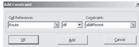
FIGURE 8.30 After adding the alldifferent constraint, Route (D22:P22) and C23:Q23 show the route from Seattle to the other 13 American League cities and back to Seattle that has been obtained by Evolutionary Solver.
