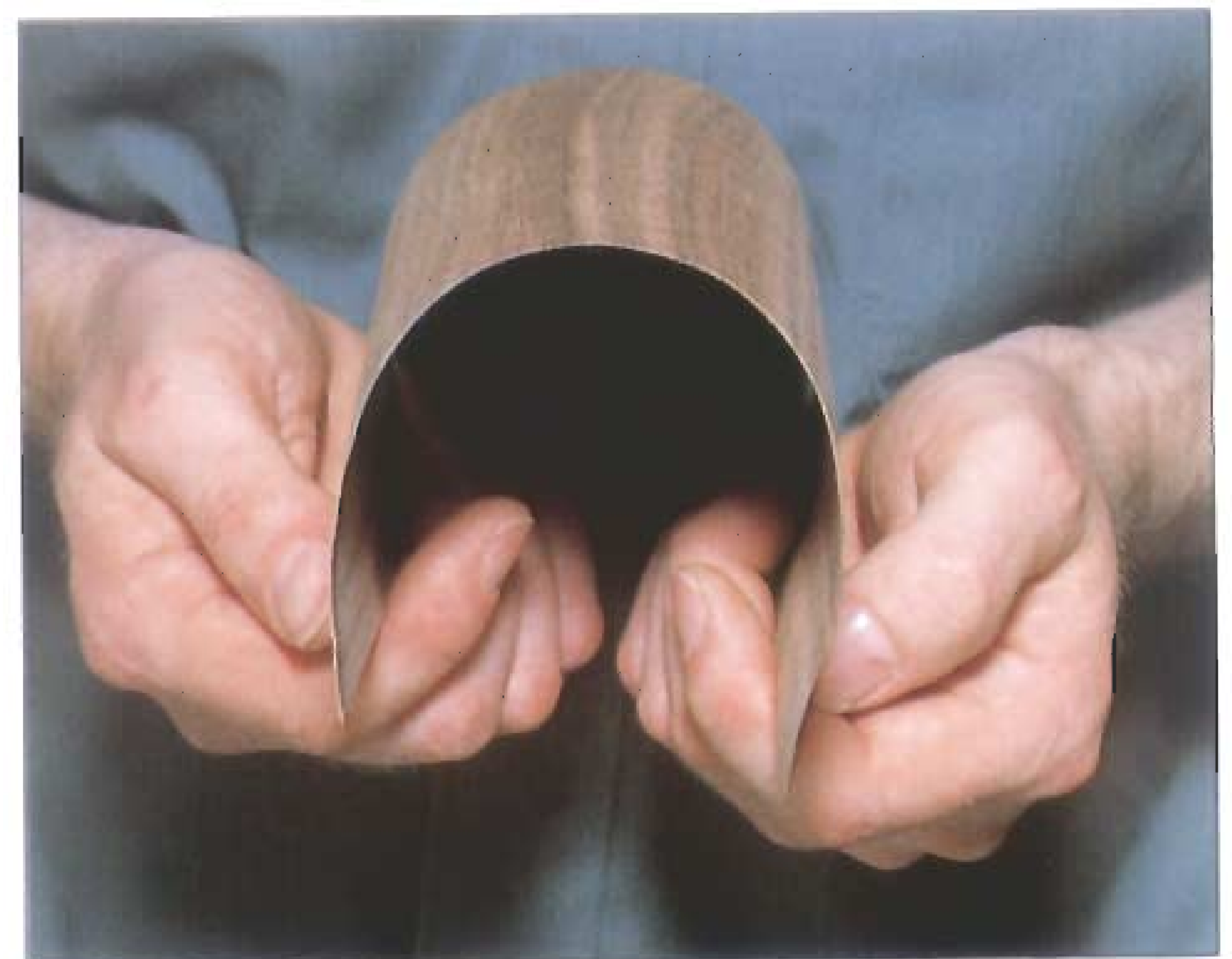
Veneers bend easily when the face side is uppermost.
