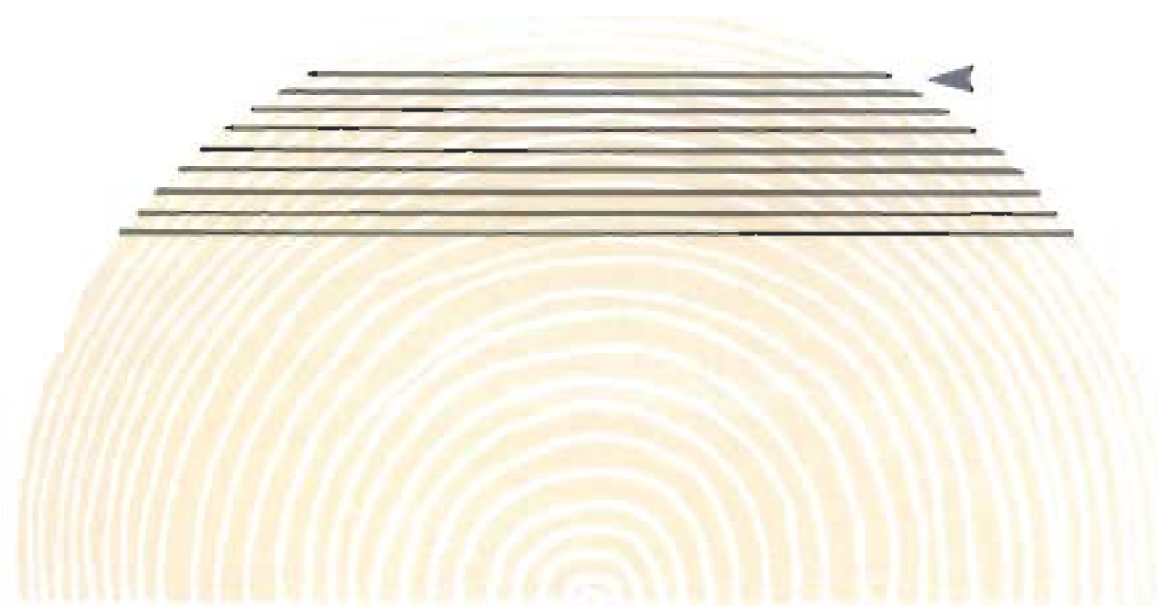
Crown cutting takes flat slices across the width of a log.
