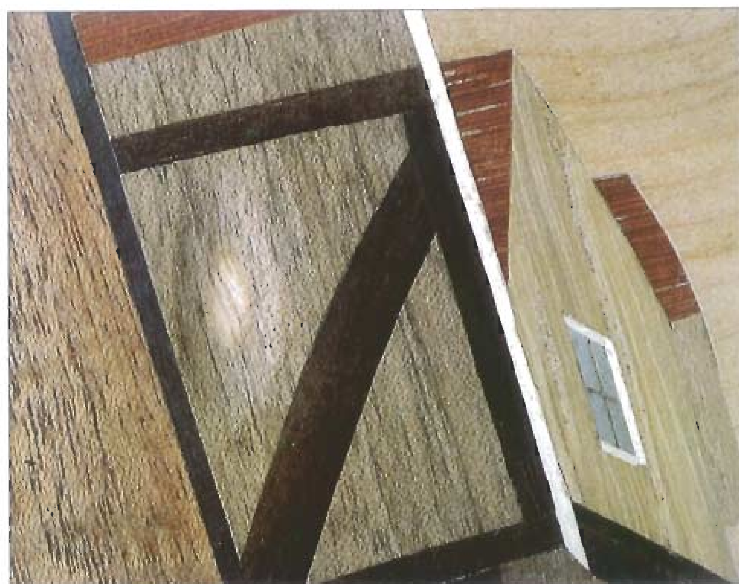
Sanding over a slight blister wears through the veneer.
