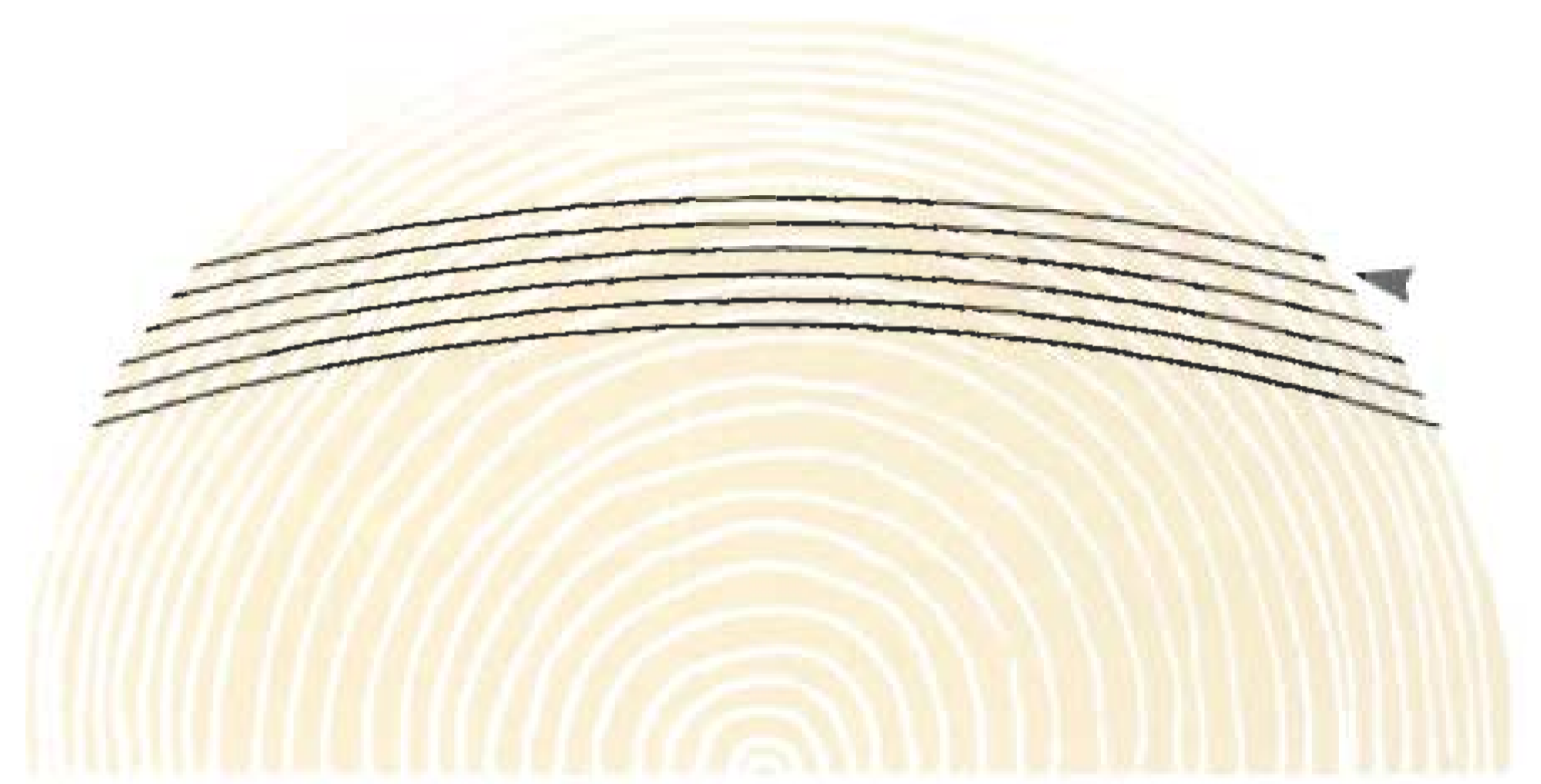
True half-rotary cut takes the first slice from the sapwood side of a log.
