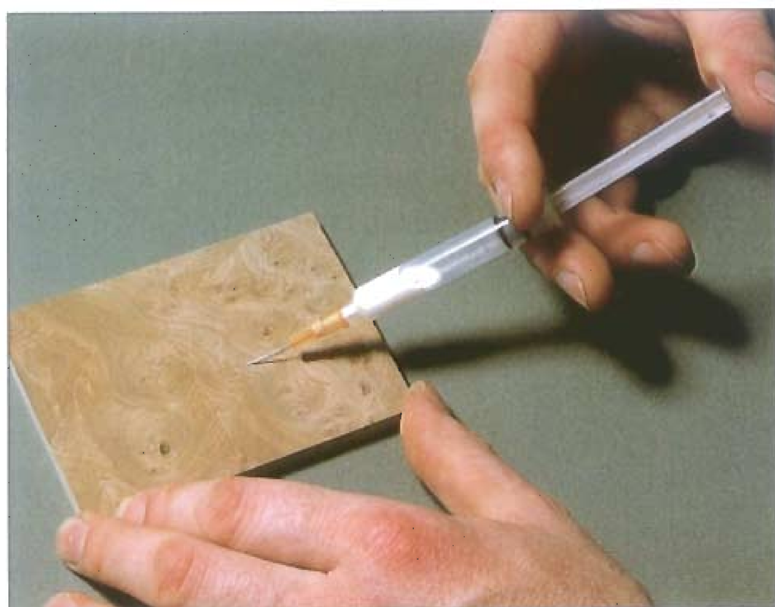
Use a syringe to insert glue under the blister.
