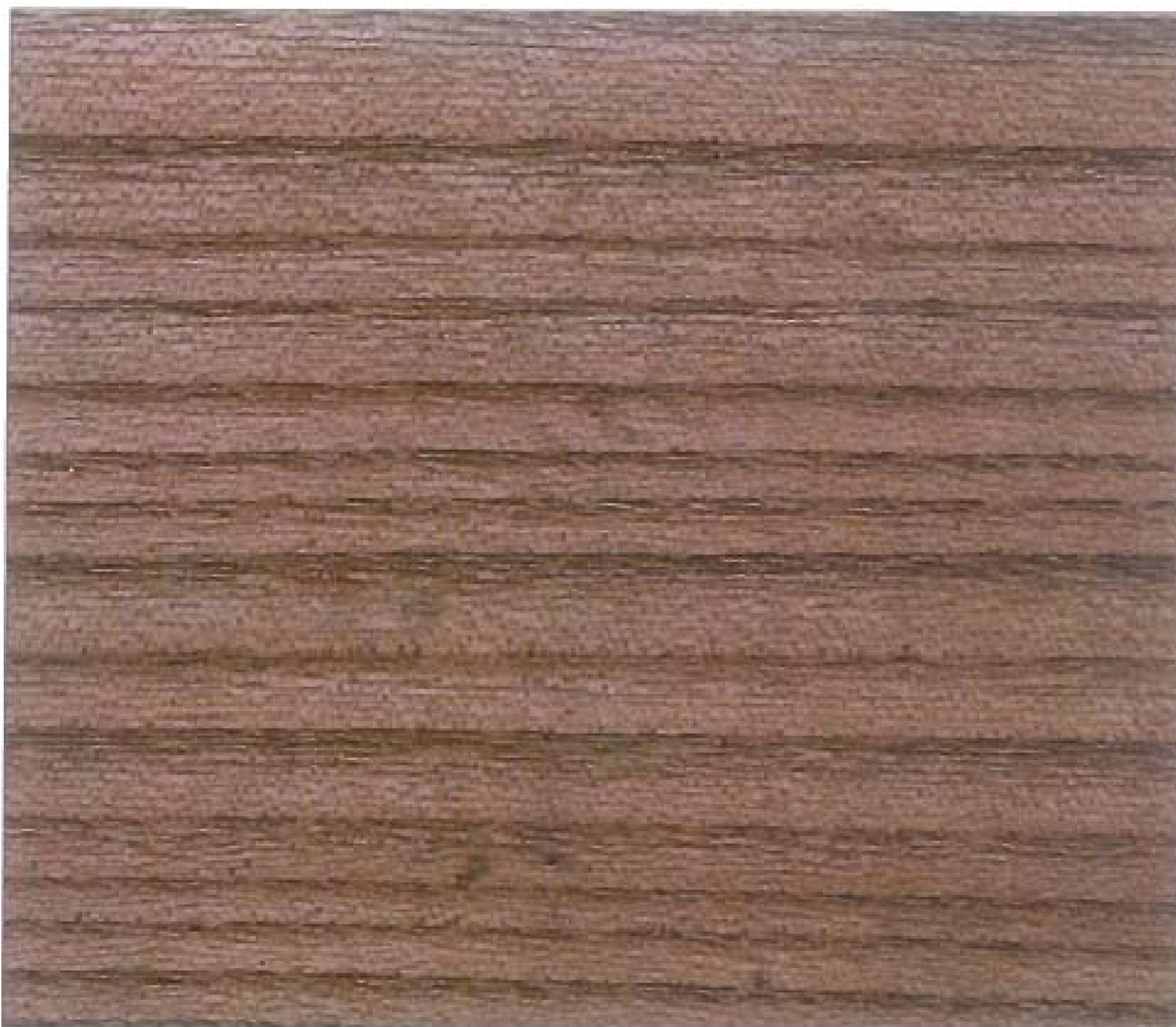
Elm veneers are produced by crown cutting.
