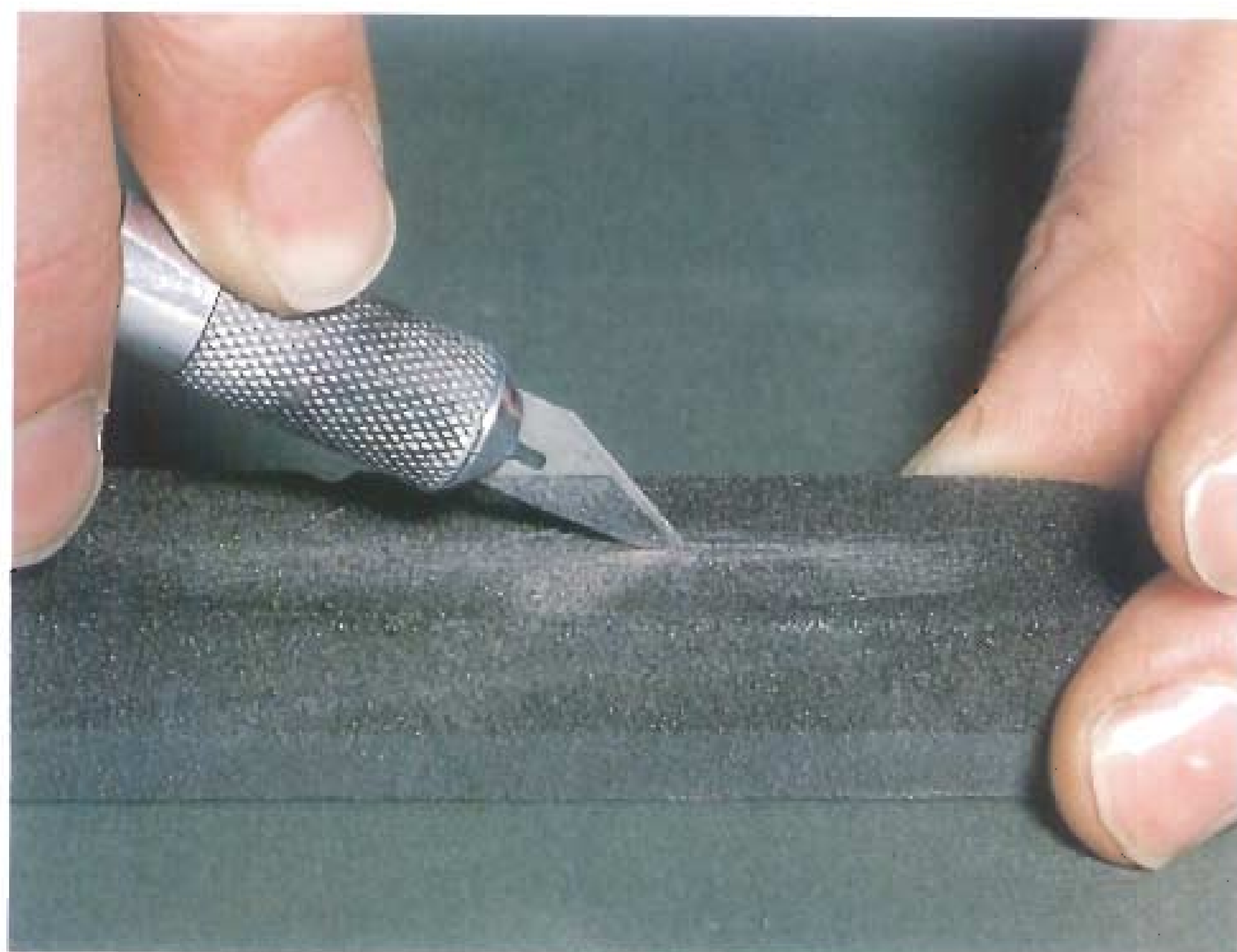
Grind the back of the blade to keep it sharp.
