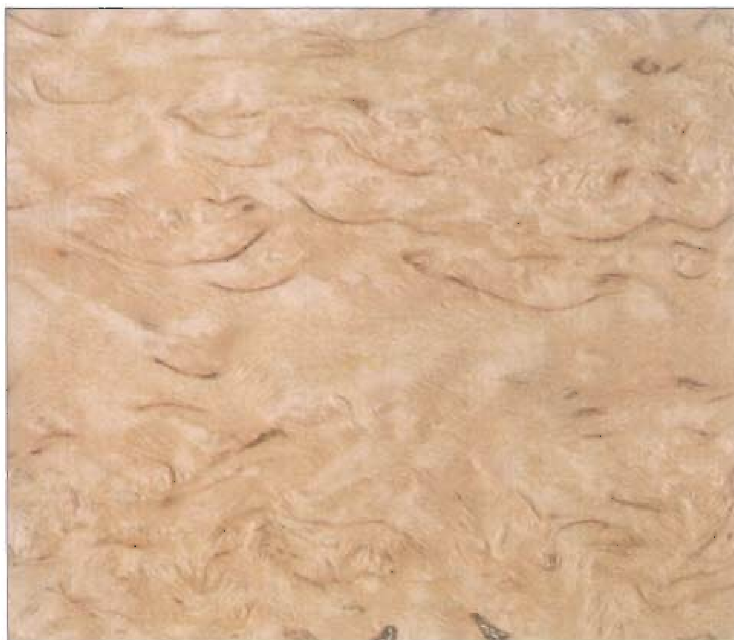
Mazur birch is produced by a rotary cut.
