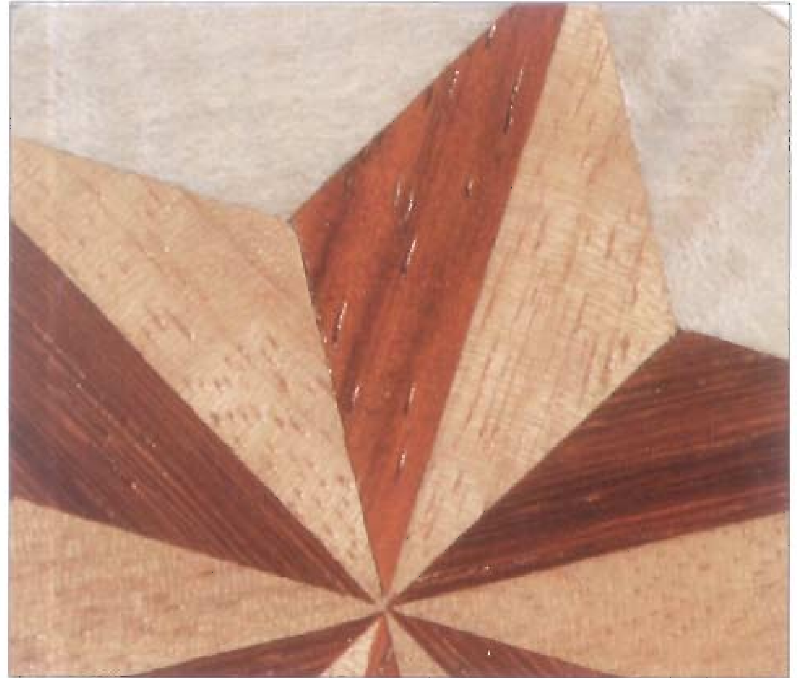
The surface of this coaster has sunk and exposed the grain details. It must be sanded and finished again.
