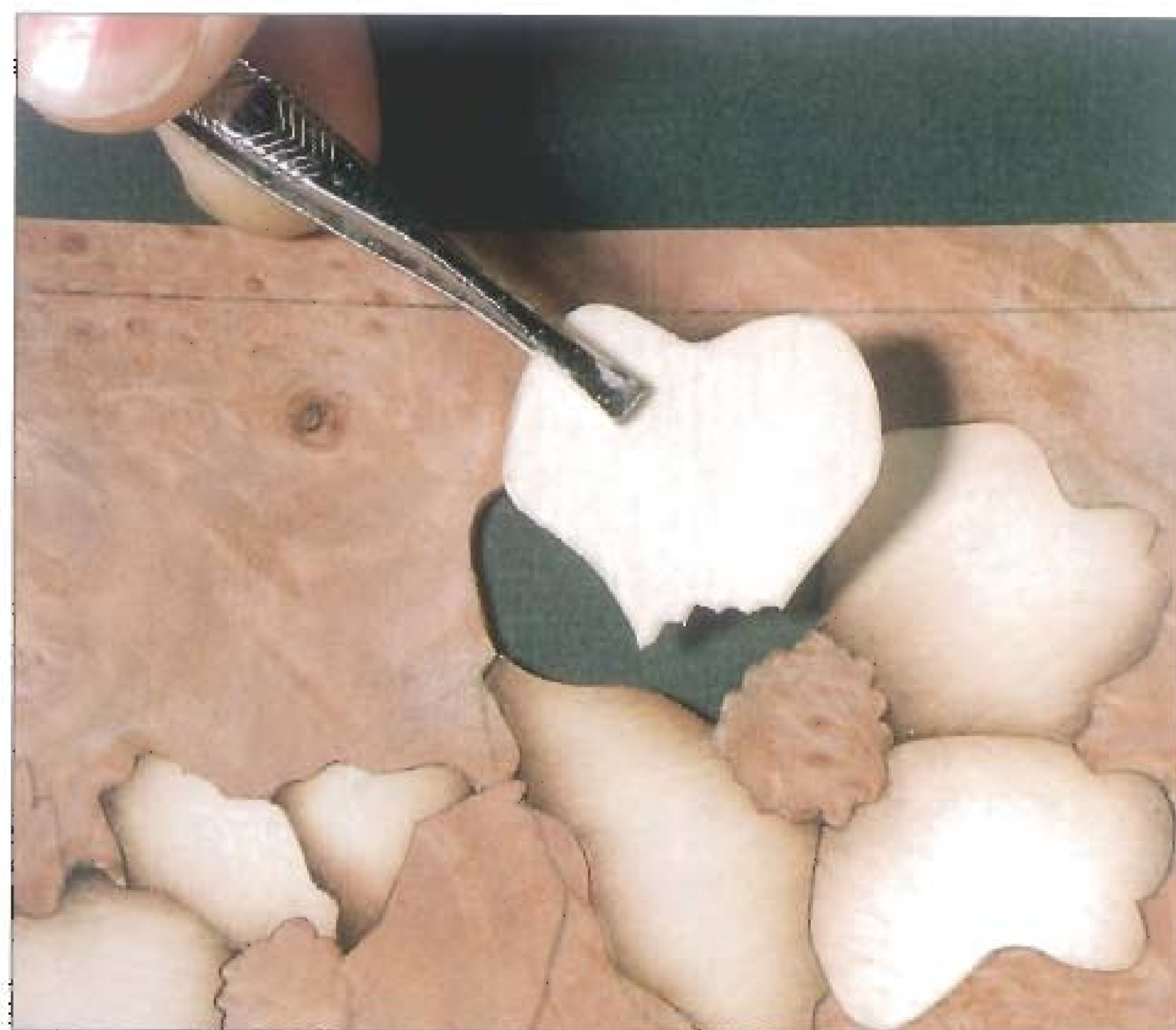
Shade a piece of veneer that is slightly larger than the window and then trim to fit.
