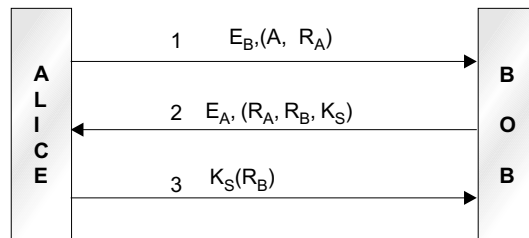
Fig. 9.13 Mutual Authentication using Public Key Cryptography
