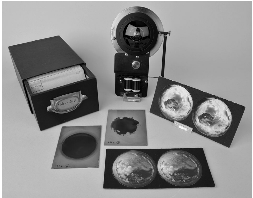
Figure 12.1 A selection of photographs taken by Hill and preserved with his cloud cameras in the Whipple Museum. Image © Whipple Museum (Wh.4416).
