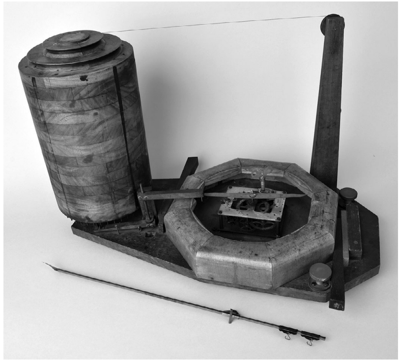
Figure 5.2 A self-recording auxanometer for measuring plant growth, made by Horace Darwin in 1876. Image © Whipple Museum (Wh.2766).
