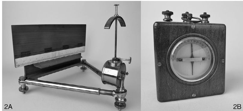
Figure 7.2 Exhibit 2A: a moving-magnet reflecting galvanometer by Elliott Brothers, 1875. Exhibit 2B: a moving-magnet pointer galvanometer, c. 1880. Images © Whipple Museum (Wh.0939; Wh.3090).
