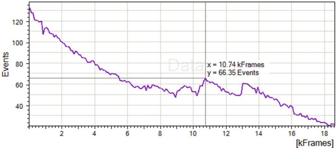
Fig. 3 Typical histogram of the number of localizations per frame for the Alexa Fluor-647 dye. The curve is built using blocks of 100 frames each for smoothing reasons. Note increases in the number of localizations (middle part of the graph) due to an increase in the intensity of the “backpumping” with a 405-nm laser. Exposure time is 50 ms/frame, detection threshold is 80 photons/pixel; 18,620 frames with 1,161,303 events were analyzed. The analysis was done in the Leica LAS AF software
