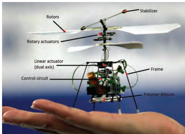
Figure 3.11 Lightest robot copter and its architecture [88].
