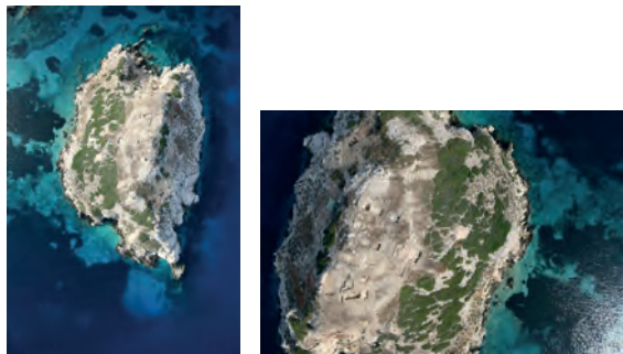
Figure 6.12 Because of the steep terrain, digital terrain models (DTMs) were created for each individual strip and merged afterwards. In addition, the DTM was edited for errors. The cell width varies between 0.5 and 3 m and the general mass point quality was 80%.
