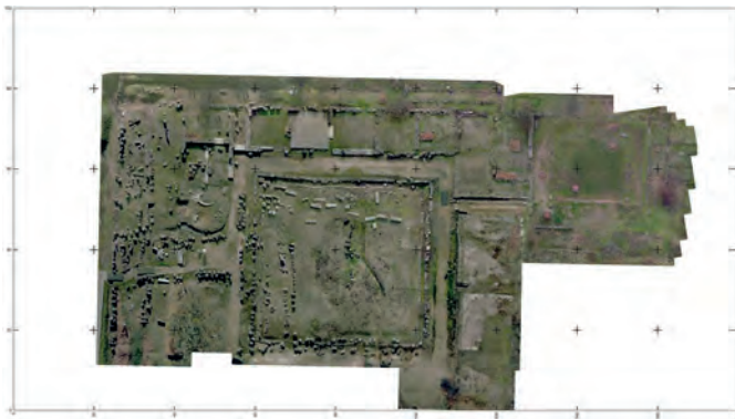
Figure 6.5 The produced orthophotomosaic with pixel size of 1 cm (acceptable results for mapping at 1:100 scale).
