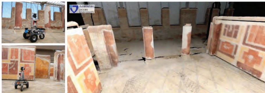
Figure 4.16 Left: Irma3D in Ostia Antica. Right: Resulting 3D model.
