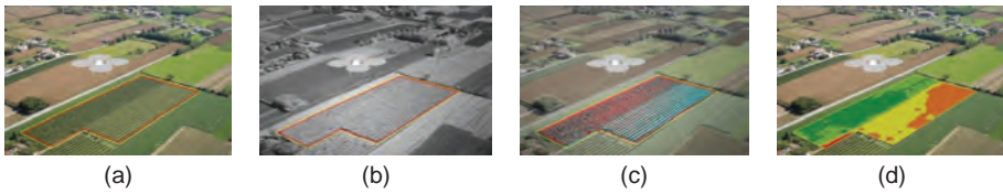
Figure 6.31 (a) The studied vineyard area, seen in (b) the NIR domain and (c) with false colour. (d) Estimated NDVI index.
