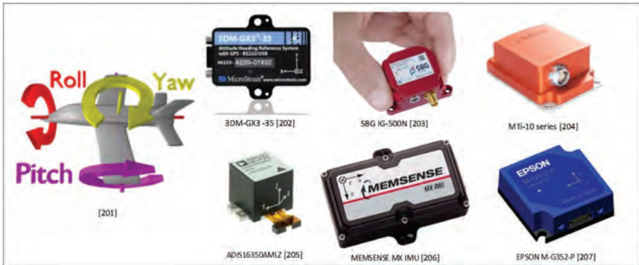
Figure 3.17 Different types of IMUs.
