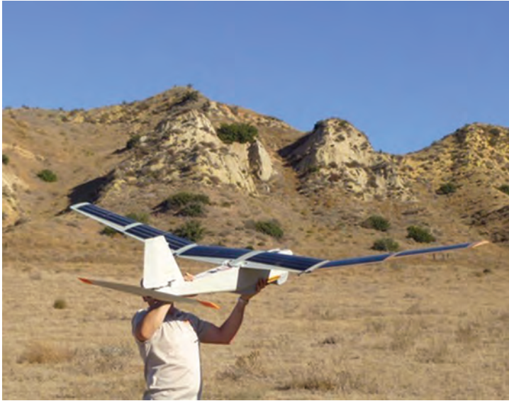
Figure 1.6 Solar-powered small UAS.
