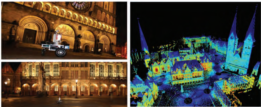
Figure 4.15 Left: Irma3D in downtown Bremen. Right: 3D model with mapped colour-coded temperature information.
