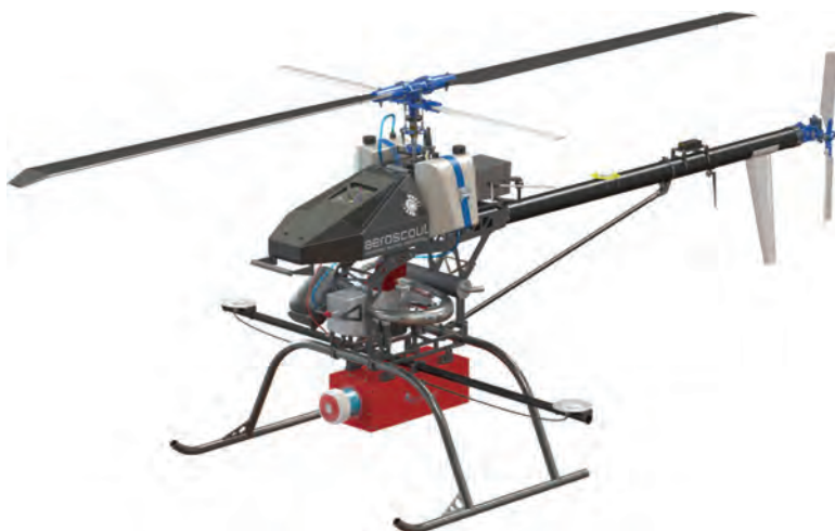
Figure 7.17 Fully integrated UAV system with the RIEGL VUX-1 laser scanner provided by Aeroscout [4].
