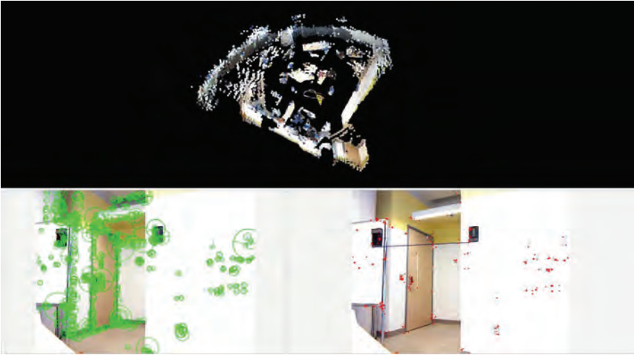
Figure 2.15 Top: Map (RGB point cloud) being created. Bottom right and left: SIFT image feature (red dots) and their scales (green circles), respectively.
