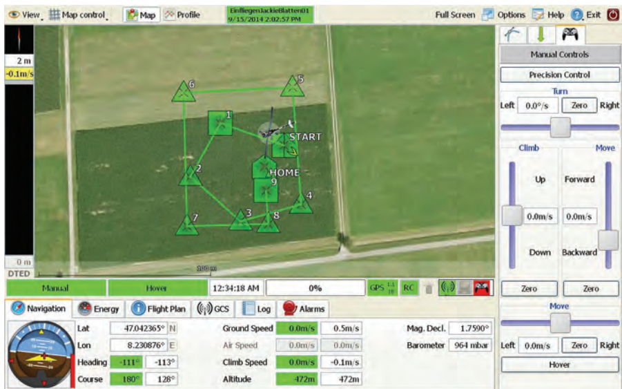
Figure 7.12 Ground control station software provided by weControl [19].
