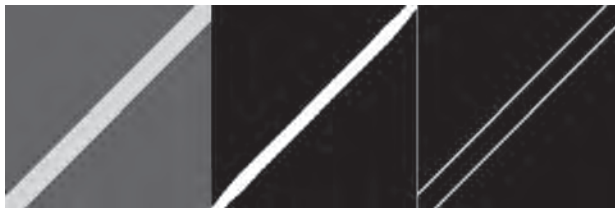
Figure 6.69 Results of linear feature detection for a synthetic image: (a) Original input image; (b) Output image with the line detection algorithm developed here; (c) Output image using line detection with EDLine.
