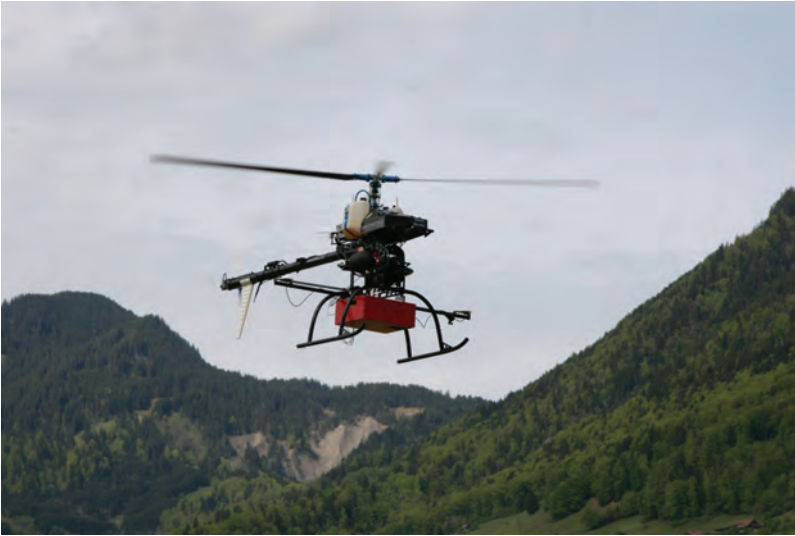
Figure 7.4 Scout B1-100 UAV helicopter [4] with onboard laser scanner and high-accuracy inertial measurement unit (IMU)/DGPS (differential GPS) navigation unit [13].
