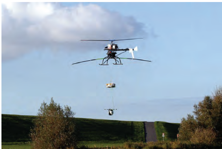
Figure 7.25 Possible bird solution of a payload integrated on the Scout B1-100 from Aeroscout.
