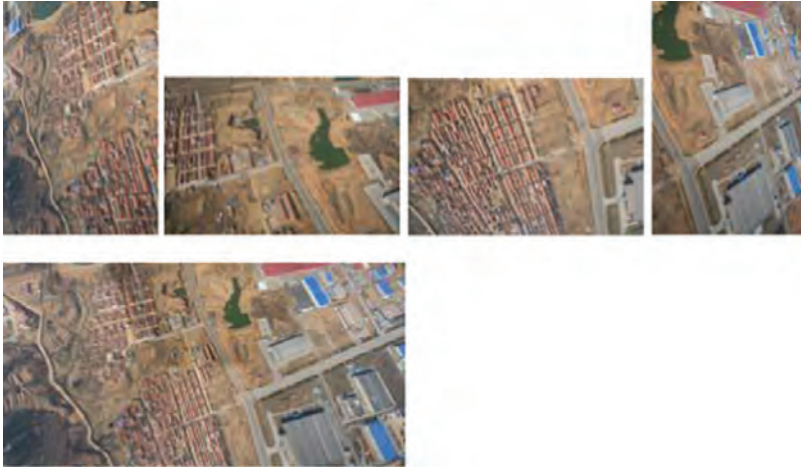
Figure 6.47 The respective images taken from each camera and the equivalent result after merging.
