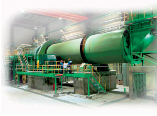
Fig. 4.10 Drum pulper with a single drum body incorporating slushing and coarse screening (source: Andritz).
