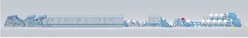
Fig. 6.81 Schematic of a state-of-the-art paper machine for LWC paper production (source: Voith).
