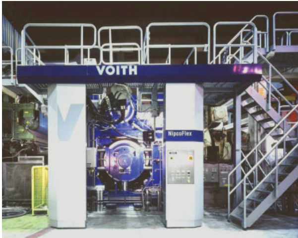
Fig. 6.73 Extended nip calender, schematic and photo of mounting (source: Voith).
