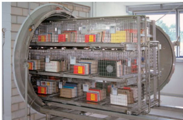
Fig. 13.6 Chamber of the Papersave Process ® mass deacidification plant with a capacity of 60 tons per year.
