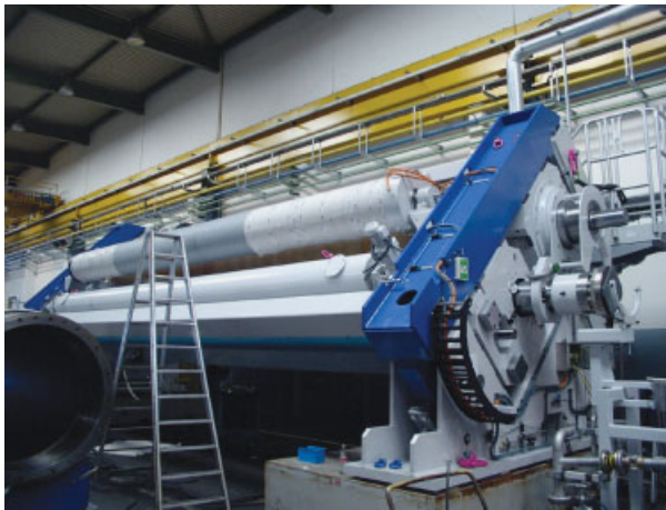
Fig. 6.71 Softcalender, schematic and photo of mounting (source: Voith).
