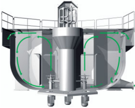
Fig. 4.37 Schematic arrangement of the Metso OptiBright™ MC flotation cell (source: Metso Paper).
