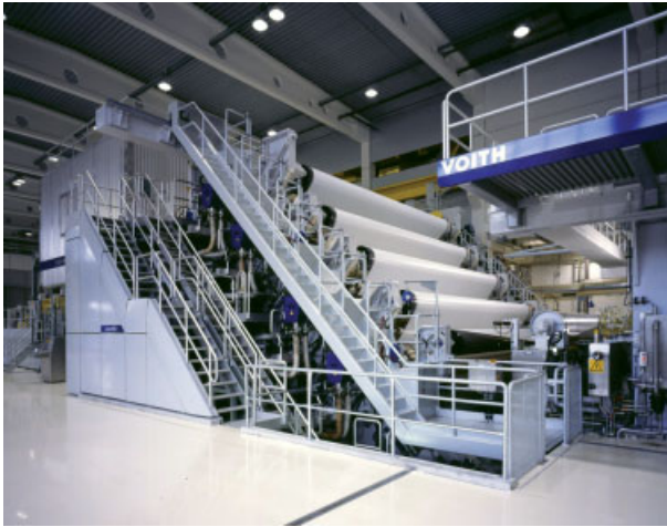
Fig. 6.72 Multinip-calender with inclined layout, schematic and photo of mounting (source: Voith).
