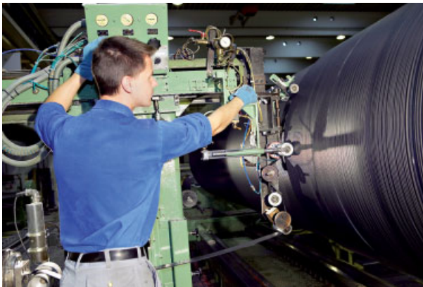
Fig. 6.10 Extrusion of rubber cover (source: Voith).
