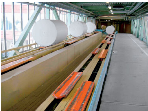
Fig. 8.20 Carousel conveyor (source: Raumaster).
