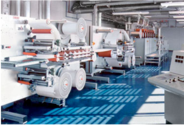
Fig. 13.8 Paper splitting machine in the Center for Book Conservation in Leipzig.
