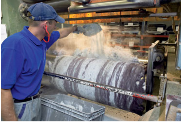
Fig. 6.9 Rubber compounding on an open mill (source: Voith).
