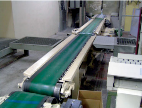
Fig. 8.18 Belt conveyor (source: Voith).
