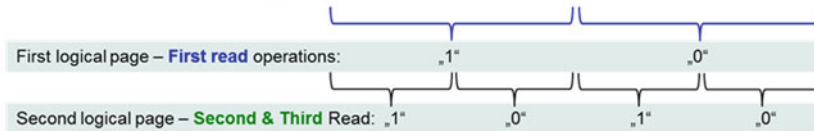
Fig. 2.86 Multi Level Cell [MLC] principles—coding scheme for two logical pages
