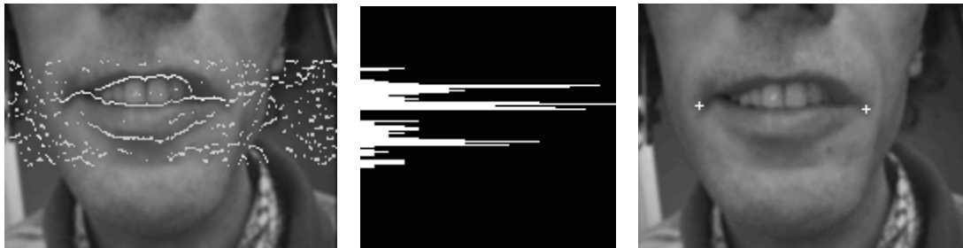
Figure 6. Mouth corner detection. From left to right: vertical minima (minima in grey, extrema in white) on a grey level image; the corresponding counting per row; mouth corner position for an open mouth
