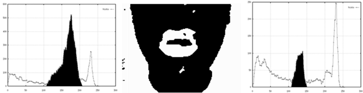
Figure 2. Lips and skin hue mode. From left to right: histogram of hue image (In black: overlap between lip and skin distribution); the corresponding segmentation of skin hue (In black); histogram of hue image when the skin mode is discarded (In black: the lip mode)
