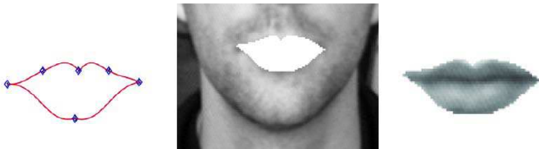
Figure 4. A lip spline, mouth image and segmented mouth area after the EM algorithm based on performance parameters. ©2008 Shafiq ur Réhman. Used with permission.
