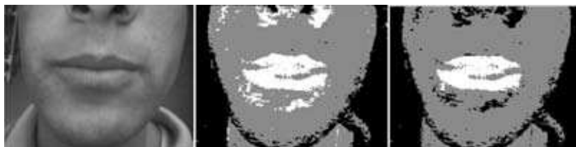
Figure 10. Lip segmentation example from (Gacon, 2005), from left to right, input image, classified pixels, classified pixels after noise reduction
