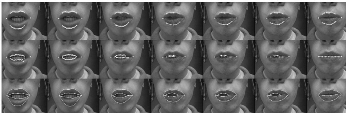
Figure 10. Lip contours extraction from seven consecutive frames. Top: outer lip contour initialisation points; Middle: inner lip contour initialisation points; Bottom: final lip contours
