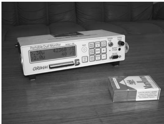
FIGURE 5.6 The Grimm 1.108 laser particle counter provides 1-minute particle counts in 14 size ranges. In this photograph, the display shows a count of 42,360 particles/L in the sizes above 0.3 micrometers and 40 particles/L above 2 micrometers. The instrument stores its readings in a memory card located underneath the display window, and the time series of 1-minute counts for 14 sizes can be downloaded by cable into a personal computer.
