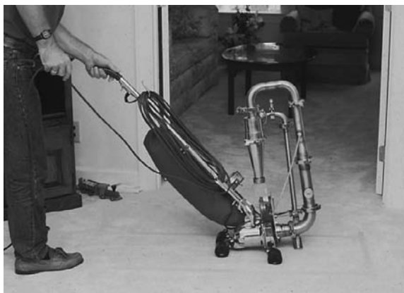
FIGURE 14.1 Special purpose vacuum, the HVS3, designed to collect a large quantity of dust in a standardized manner for laboratory analysis of the sample's chemical composition and pollutant concentration. (Courtesy of Dr. Robert Lewis, USEPA; see also Chapter 15 and Figure 15.4.)
