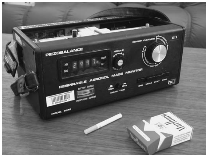
FIGURE 5.7 Kanomax 8510 piezoelectric microbalance (Piezobalance) for measuring particle mass concentration at 1-minute or 2-minute averaging times. In this photograph, the display reads “2997” momentarily to show the user the initial starting frequency of the piezoelectric crystal. An internal size impactor is installed inside the instrument to allow it to measure either PM_{2.5} or PM_{3.5} respirable suspended particulates (RSP) mass concentrations.
