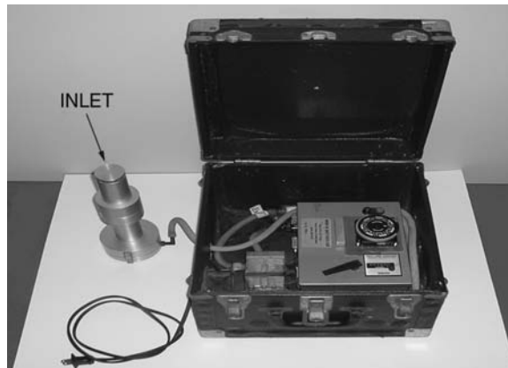
FIGURE 5.3 Harvard impactor (HI), also known as the Black Box. Shown is a PM_{2.5} nozzle. The HI is programmable using the timer to collect data automatically for specified periods up to 2 weeks.
