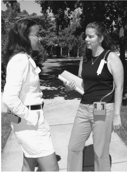
FIGURE 15.3 Open-face air sampler (left) and sampler with size-selective inlet (right) in use for personal exposure monitoring. (Courtesy of persons in the photograph.)
