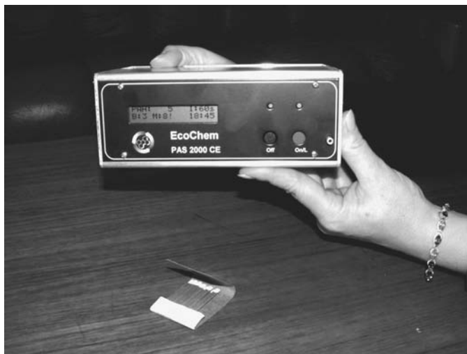
FIGURE 5.9 EcoChem PAS 2000 CE photoionization monitor for measuring the mass concentration of fine particulate polycyclic aromatic hydrocarbons (PPAH). The display shows a current PPAH concentration reading of 5 \text{ ng/m}^3 , the sampling time setting of 60 sec), a code for the battery life remaining (B = 3), a code for the memory used (M = 8), and the clock time of 18:45.
