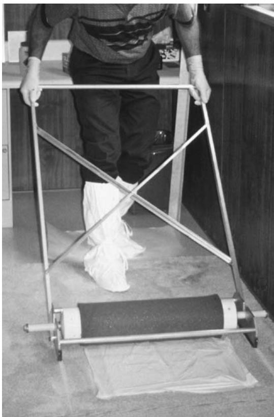
FIGURE 15.8 California roller in USEPA custom sled designed to eliminate influence of user on applied pressure.
