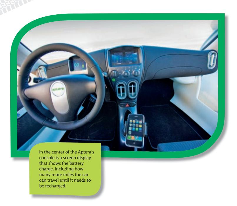
The Aptera's dashboard is modest compared to that of other cars, but it offers enough gadgets and information to satisfy any car buff or technology geek. The Aptera offers smartphone connectivity and a GPS unit. There is also an efficiency meter that allows the driver to see how much energy is used as he or she drives. And, since the car is electric, a simple power button turns the car on and off.
