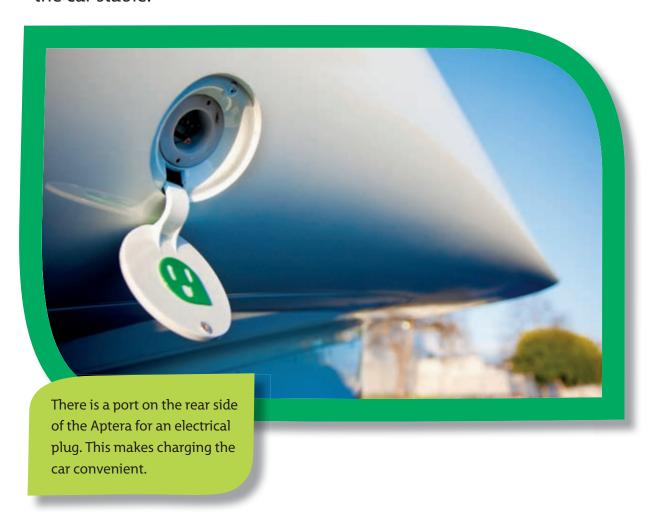
The batteries can be recharged by plugging the Aptera into a regular wall outlet like those in your house. If you use a standard 110-volt outlet, the batteries can be fully recharged overnight, but if you plug it into a 220-volt outlet (like the outlets used for electric washers and dryers), it will take only four hours to give the car a full charge.
