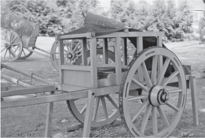
Fig. 4.3 Artillery forge Fort Ligonier. (Photo by the author.) Forbes's artillery train would have included at least one of these portable forges, allowing Royal Artillery artificers to make necessary repairs and spare parts. Freight wagons would have hauled the tons of charcoal needed to feed the forge.
