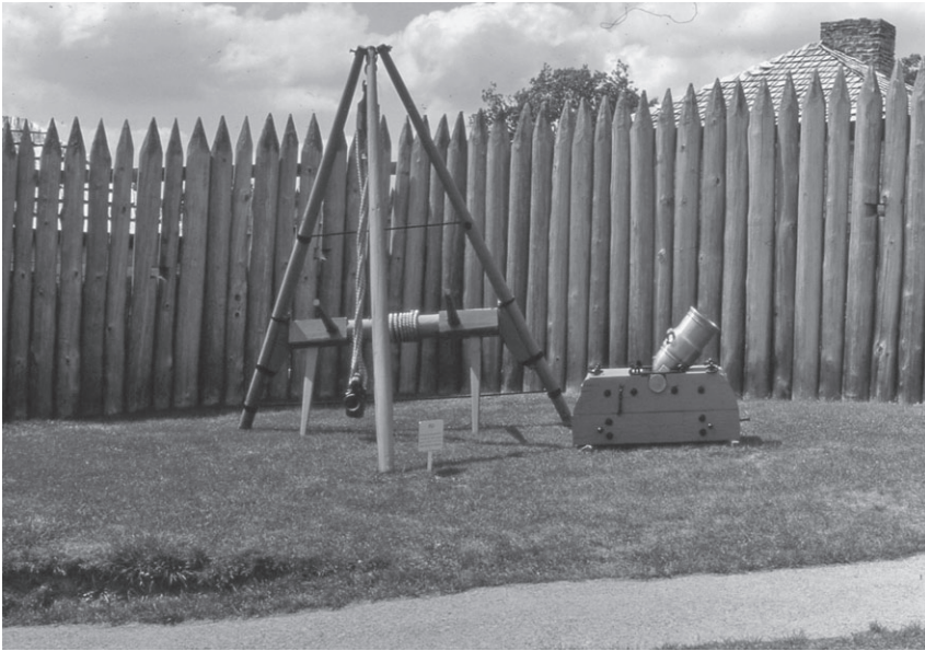
Fig. 4.2 Artillery gin and coehorn mortar, Fort Ligonier. (Photo by the author.) The gin, used in lifting heavy artillery tubes onto their carriages, was just one item in the vast store of materials under the control of Captain-lieutenant David Hay's Royal Artillery. The coehorn mortar, designed to fire explosive shells into an enemy fortification, would have been the workhorse of any siege batteries erected against Fort Duquesne.
