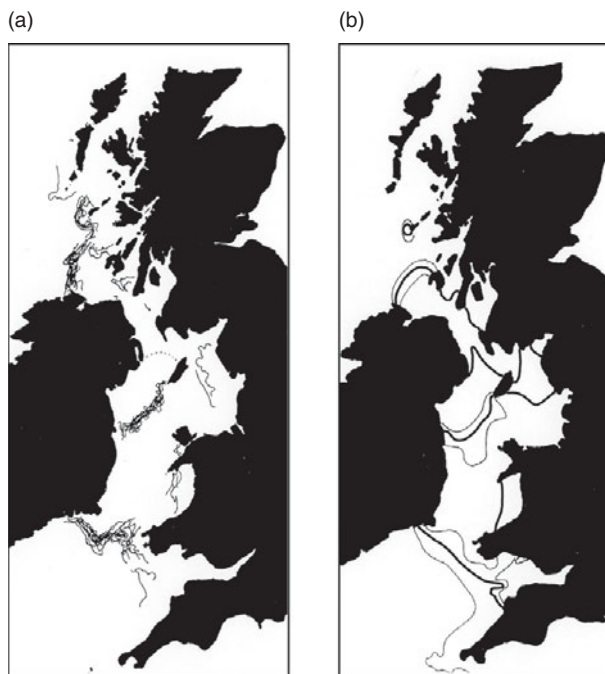
Figure 8.2 (a) Composite of frontal positions from clear images for the period May–September 1980, and (b) contours of SH from a numerical model showing the predicted frontal positions at SH = 2.7 (thick lines) and the extent of the transition zone (thin lines) defined by \Delta SH = \pm 0.5 . After Simpson and James, 1986, courtesy of the American Geophysical Union.
