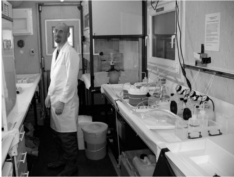
Figure 5.3 The interior of the radioisotope laboratory aboard RRS Discovery , Celtic Sea, June 2010. The laboratory, part of the UK National Marine Facilities, is installed within a standard shipping container so that it can be installed on different research vessels as required. (Photo by J. Sharples.)
