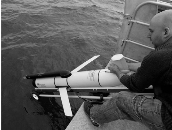
Figure 1.9 Deploying a glider into the Irish Sea. The conductivity and temperature sensors are just visible underneath the left wing. The black tube on top is a turbulent dissipation instrument, with the shear sensors visible forward of the glider nose. (Photo courtesy of the National Oceanography Centre, UK.)
