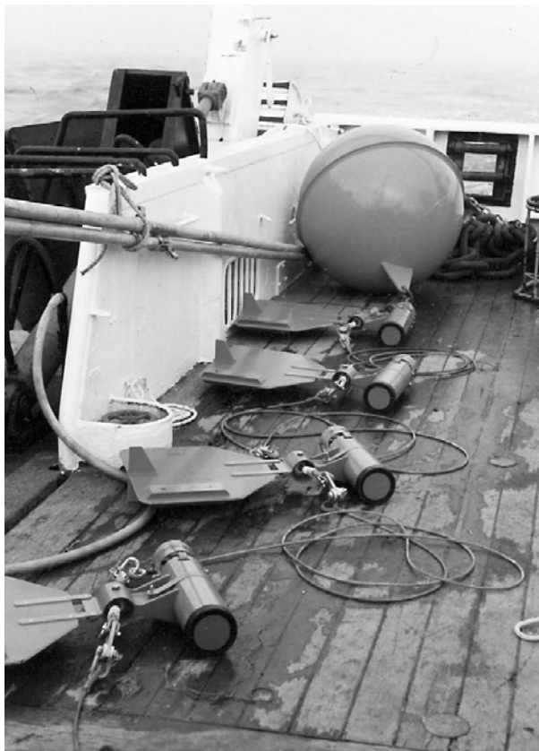
Figure 1.7 A mooring ready for deployment in the eastern Irish Sea (depth about 35 metres). The instruments are Aanderaa recording current meters (RCMs), which use a rotor with the large vane aligning the instrument to the flow. The large spherical buoy (about 1 metre diameter) stretches the instrument line upward from an anchor on the seabed. Each RCM also had temperature and conductivity sensors to provide a coarse vertical profile of salinity. (Photo by J. Sharples.)
