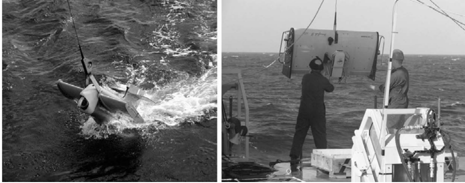
Figure 1.5 Two examples of towed, undulating vehicles that we have used in shelf sea research. Left: Seasoar, looking like a short, stubby-winged aeroplane. Right: Scanfish, a relatively simple wing-shaped vehicle that incorporates a downward-looking echosounder used for automated seabed avoidance – a very useful feature when working in shallow seas. (Photos by J. Sharples.)
