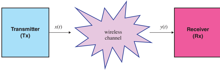
Figure 2.1 A wireless communication system consisting of three parts
