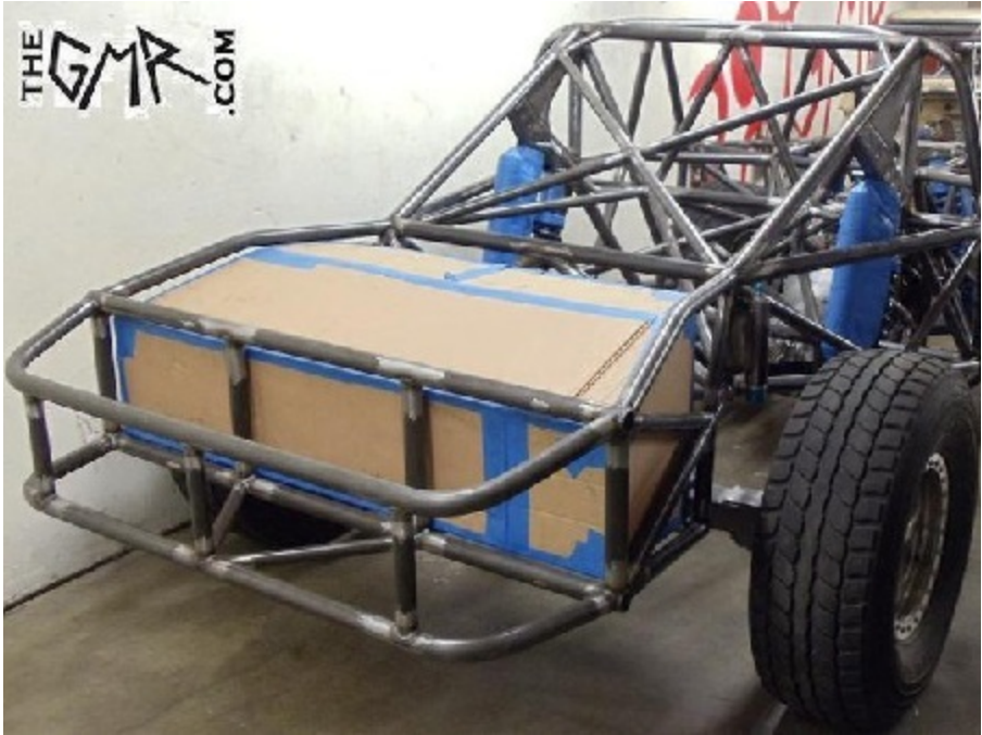
The first TIME this truck is sitting on its wheels under its own weight, the tube work is almost done along with the shock / chassis components. I was able to bolt on all the suspension and use some springs from the Hummer H1 to get her rolling around..
