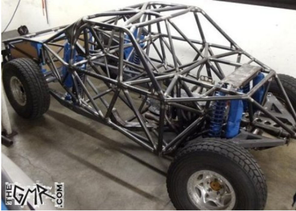
The first TIME this truck is sitting on its wheels under its own weight, the tube work is almost done along with the shock / chassis components. I was able to bolt on all the suspension and use some springs from the Hummer H1 to get her rolling around..
