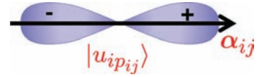
Figure 7.3: The angular dependence of a p orbital. Here it is identified as |u_{ip_{ij}}\rangle , centered on the indexed location of an atom i and along a direction \alpha_{ij} that passes through i and j .
