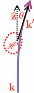
Figure 8.9: Quasielastic angle-dependent scattering such as with acoustic phonons in valleys with spherical constant energy surfaces or by impurity ions.
