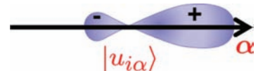
Figure 7.4: The angular dependence of an sp hybrid orbital. Here it is identified as |u_{i\alpha}\rangle , centered on indexed location of an atom i and along a direction \alpha that satisfies the hybridization condition \lambda = \sqrt{3} , \sqrt{2} or 1.
