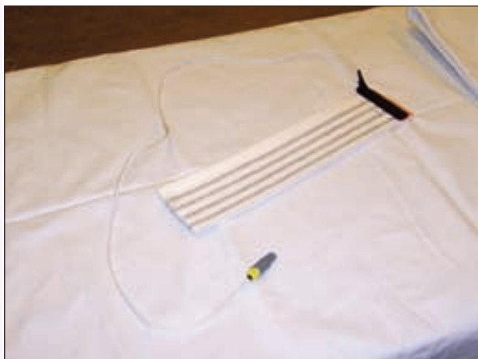
3.53 Incontinence pad with temperature-sensitive diodes.
