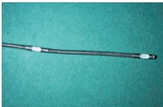
3.34 Catheter-mounted solid-state transducers.
