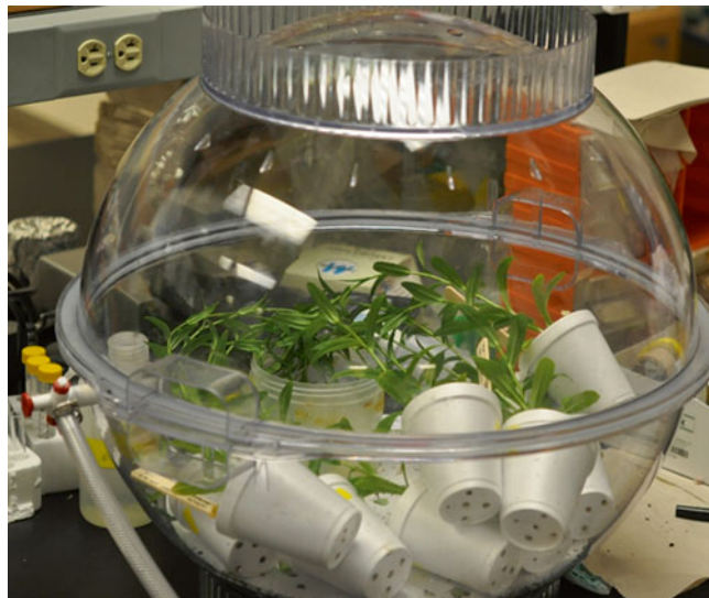
Fig. 5 Camelina floral dip transformation apparatus. A large desiccator is plugged in with a vacuum pump and a pressure gauge. The infiltration solution (with Agrobacterium ) is placed in a beaker inside the chamber. Young inflorescences are dipped inside this solution and the chamber is evacuated until the pressure of 20 psi is reached. The pressure is maintained for 5 min, after which the vacuum is slowly released
