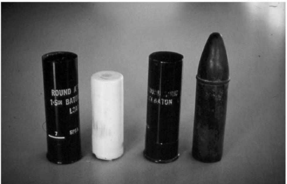
Figure 6.15 1.5 in/37 mm riot control baton rounds. The original shaped black rubber bullet was replaced by an ivory coloured plastic polyurethane bullet in an attempt at reducing the incidence of fatalities in service use in Northern Ireland.
