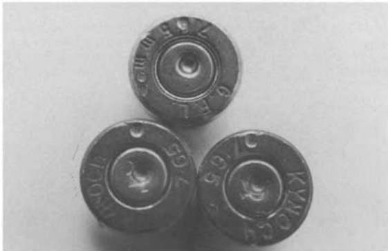
Figure 9.23 The marks left at the 12 o'clock positions on the cartridge cases indicate a selfloading pistol with a loaded chamber indicator pin. In this instance a Walther PPK.
