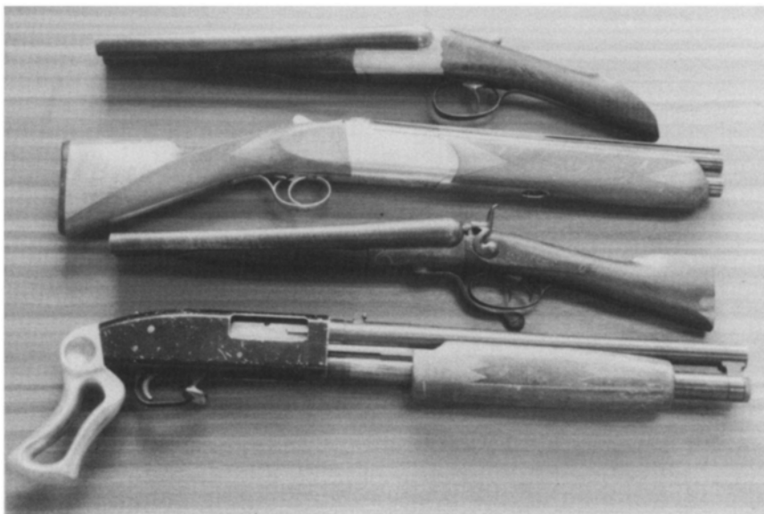
Figure 2.1 Sawn-off shotguns received at the laboratory in casework submissions. Derived from: double-barrelled side-by-side English pattern gun, double-barrelled over-and-under gun of the type commonly used in clay pigeon shooting, Jones action double-barrelled side-by-side hammer gun manufactured in the 1860–1870 period and an American Mossberg pump-action gun.
