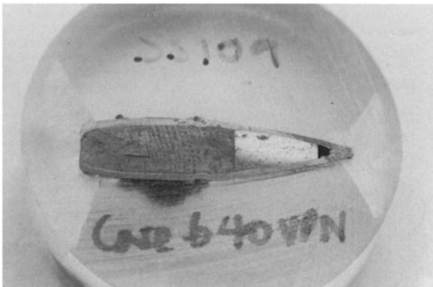
Figure 6.18 Microsection of Nato SS109 5.56 mm bullet showing truncated cone shaped hard steel core in front of the plain lead alloy filling.
