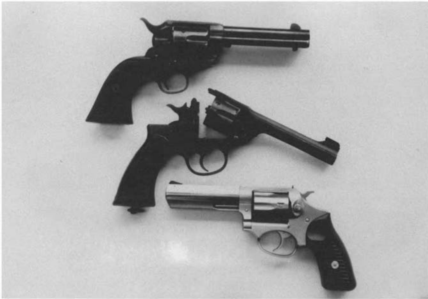
Figure 4.3 Solid-frame single-action revolver typified by the Colt Model 1873, hinged-frame Webley revolver and modern solid-frame double-action stainless steel revolver by Sturm Ruger.
