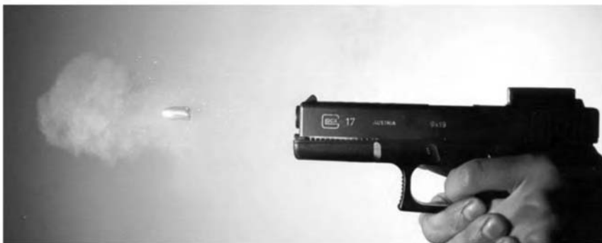
Figure 8.13 High-speed photographic image of Austrian 'Glock Model 17' 9 mm pistol being fired. Un-burnt particles of propellant can be seen travelling alongside the bullet. Such high velocity particles are capable of producing punctuate tattooing injuries in the margin of the bullet entry wound, when firing takes place at short distances and before the effects of air resistance slow them down. At this point the slide has moved back sufficiently for the breech to begin unlocking, allowing a flash to be visible in the barrel-slide gap.
