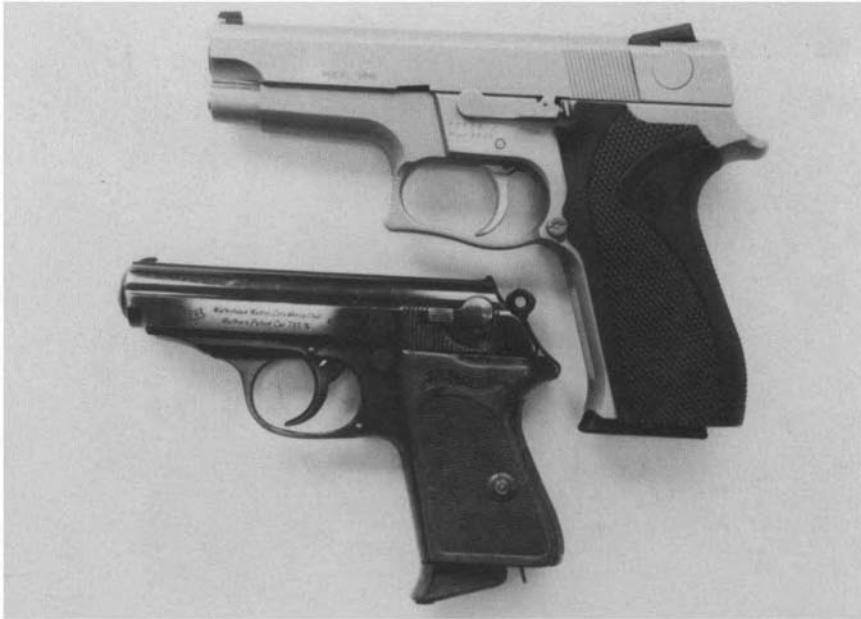
Figure 4.6 Stainless steel Smith and Wesson Model 5946 'double-action only' 9 mm self-loading pistol next to Walther PPK 7.65 mm true double-action pistol with hammer decocking safety catch.
