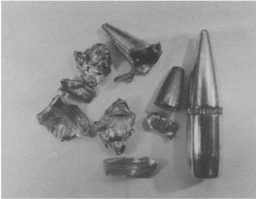
Figure 7.24 The composite form and the design of the current Nato 5.56 mm bullet loading frequently leads to missile blow-up effects at close ranges. The truncated cone steel penetrator from the core is shown in the centre right of the field.
