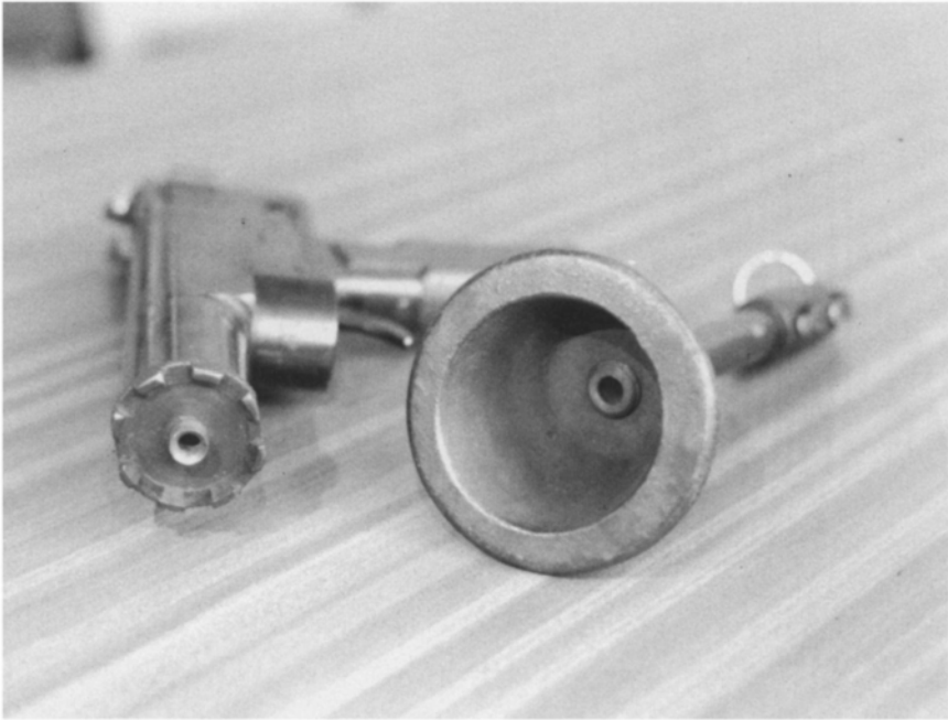
Figure 8.22 The varied geometry of the muzzle ends of humane killing devices, intended for use in abattoirs, can impart characteristic marks around the wound margins of human victims.
