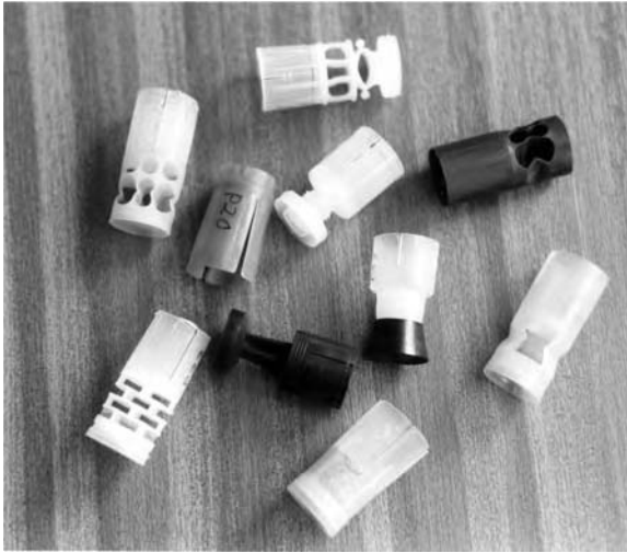
Figure 5.8 A few of the many different designs of plastic cup wads used in the loading of shotgun ammunition. The construction of the wadding has implications in respect of close range wound effects and the identification of the brand of cartridge used in an offence.
