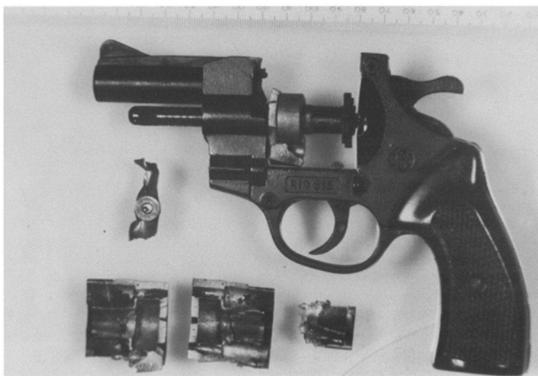
Figure 9.1 Zinc alloy blank revolvers which had their blockages drilled out to allow their use with bulletted ammunition are often capable of surviving many firings; the one shown is an exception. A remote firing device should always be used when it is necessary to test fire such weapons.
