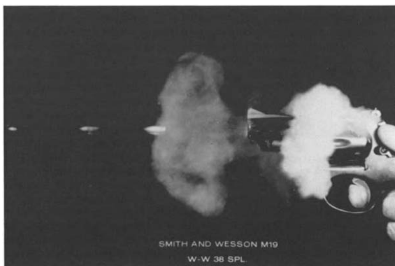
Figure 9.32 High-speed triple flash photograph of revolver being fired clearly shows the venting of discharge gases from the area of the cylinder gap. Such an effect will increase the tendency for identifiable gunshot residues to be found upon hand and face swabs and upon the clothing of the firer. The opening of the breech as the slide or bolt of a self-loading or pump-action arm is moved to the rear, will have a similar effect.
