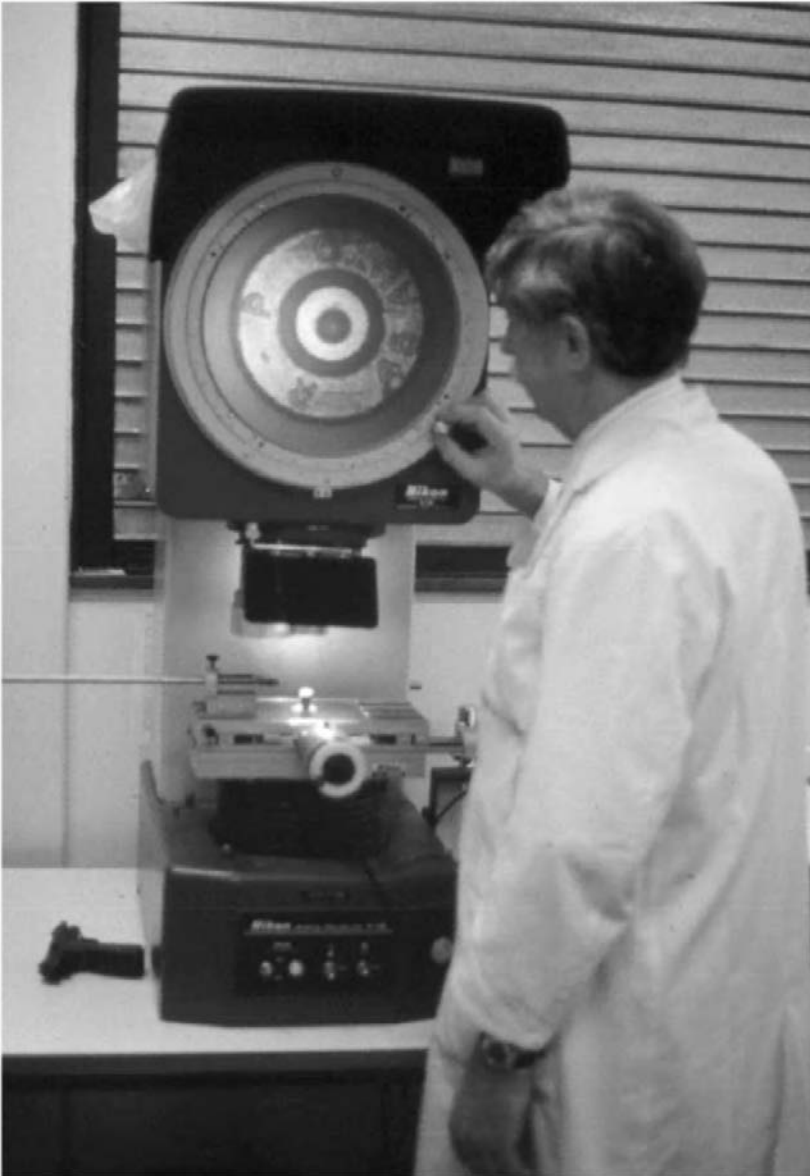
Figure 9.20 Examination of cartridge cases and bullets using the profile projector allows the majority of the information for the FBI program computer search for weapon type to be accurately recorded.
