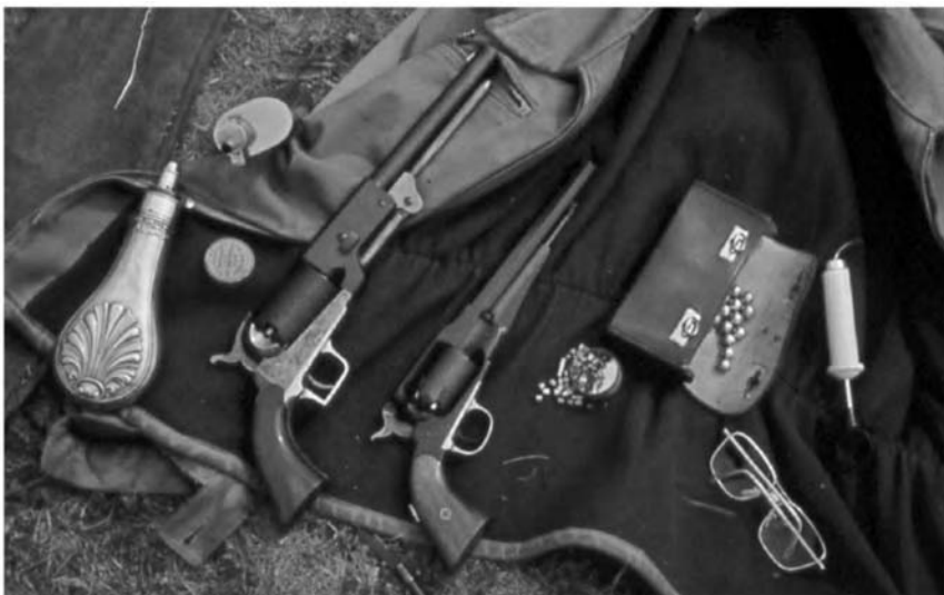
Figure 1.8 Modern Italian-manufactured muzzle-loading percussion revolvers used on a firing range by black powder enthusiasts. 1847 Colt Walker and 1861 Remington Army reproductions with powder flasks, percussion caps, .454 inch diameter cast lead balls, and lubricant grease.
