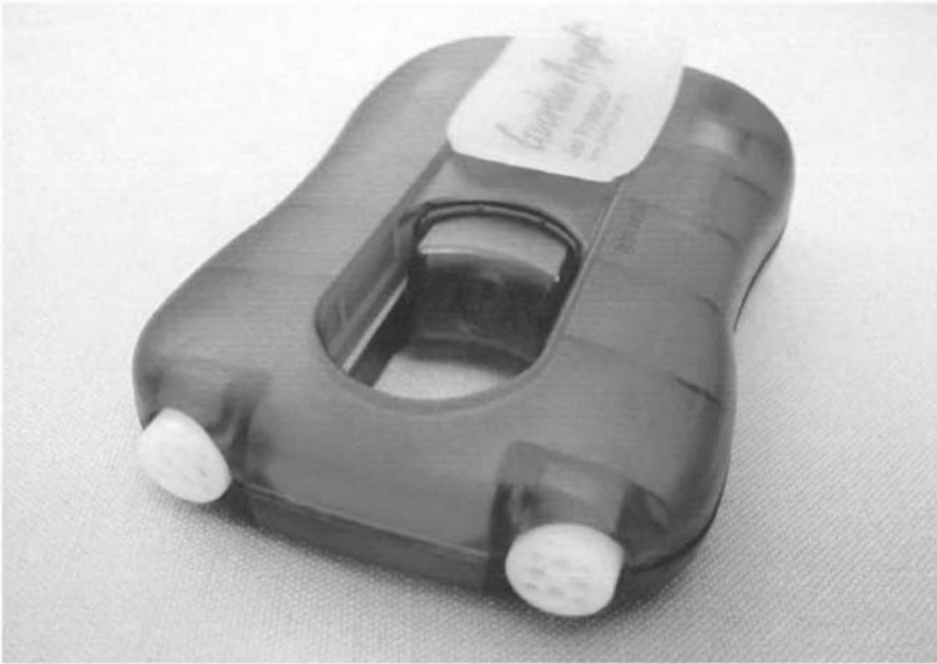
Figure 9.47 Swiss-manufactured "Guardian Angel" self-defence device. This two-shot device uses the impulse generated by the discharge of a special blank cartridge to project the capsaicin-based agent through multi-holed nozzles as a dispersed pattern over an effective range of between 1.5 and 13 feet (0.5–4m).
