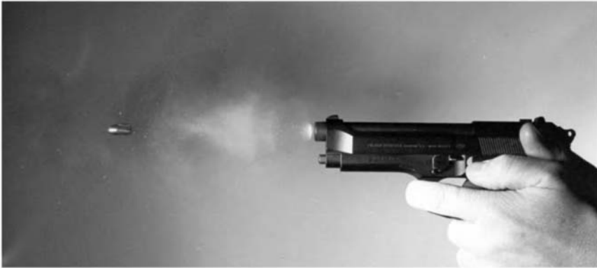
Figure 4.17 High-speed photograph of Beretta 92F 9 mm pistol being fired. At this point the slide has recoiled backwards with the barrel to the point where the breech will begin to unlock, so as to allow the slide to move to its rearmost position to cause the extraction and ejection of the spent cartridge case, followed by the return of the slide and the stripping of a fresh cartridge from its 15-shot magazine.
