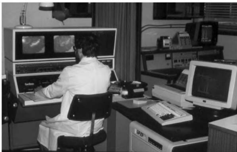
Figure 9.35 Operator at the controls of a twin screen electron microscope fitted with energy dispersive X-ray analyser.
