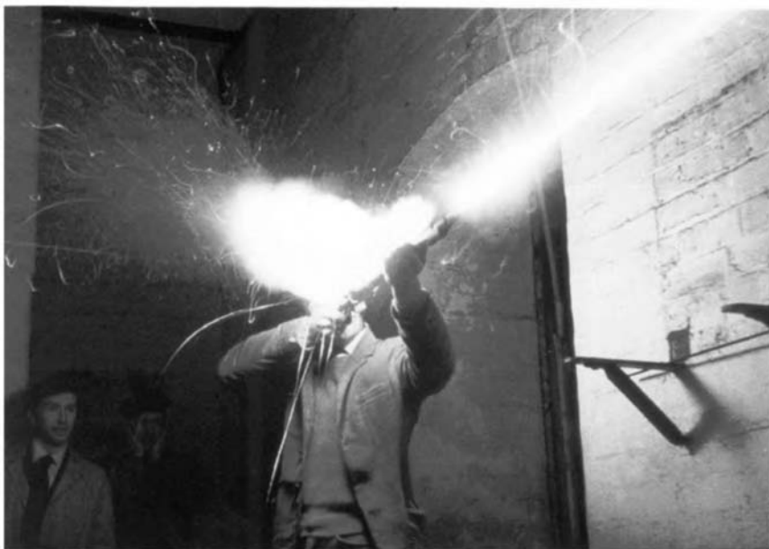
Figure 1.1 The firing of a flint-lock musket. The flash of the priming charge in the pan, which immediately precedes the firing of the main charge, provides the illumination for this picture.
