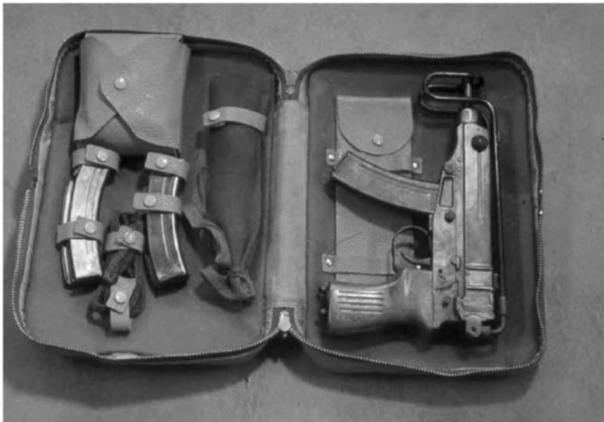
Figure 4.11 One of six cases recovered from a burnt out flat previously occupied by Middle Eastern students. Each case contained a Czech Skorpion VZOR 61 compact sub-machine gun, a holster, spares kit and package of 7.65 mm (.32 ACP) ammunition. Originally designed for tank crew, but later favoured as a concealable automatic arm for terrorist use along with the Polish WZ 63, which is chambered for the 9 mm Makarov cartridge. A Skorpion was used by the Red Brigade in the assassination of Andre Moro, the former Italian Prime Minister.
