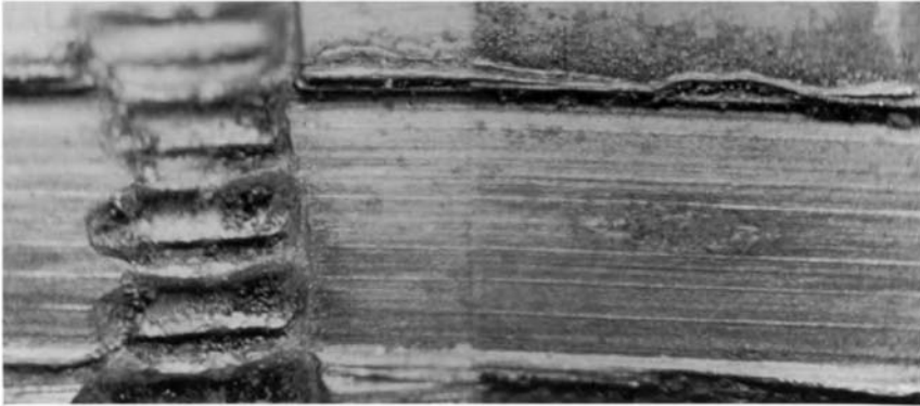
Figure 9.28 View of matching rifling land impressions on a .38 in jacketed bullet. Once the initial match point has been found the bullets are then rotated to confirm matching points around the rest of the missile's rifled exterior.
