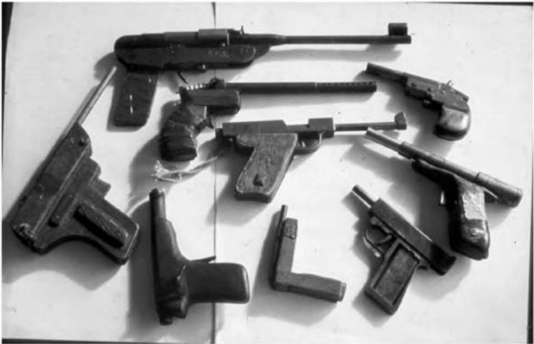
Figure 9.39 Just a few of the home-made guns (zip guns) received at the laboratory in casework submissions. The weapon shown at the top has been derived from an air weapon modified to allow the discharge of .22 in rim-fire ammunition.
