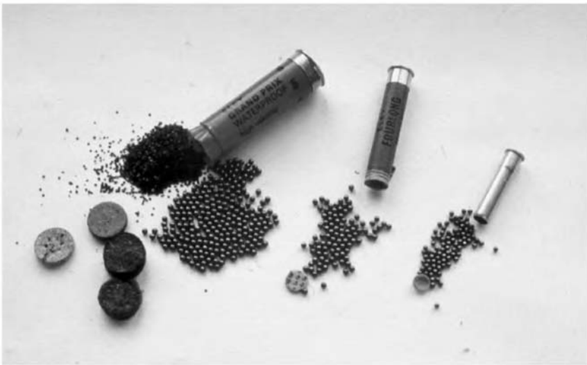
Figure 5.10 Disassembled 12 bore, .410 and 9 millimetre rim-fire shotgun cartridges loaded with conventional shot loads and fibre wadding.
