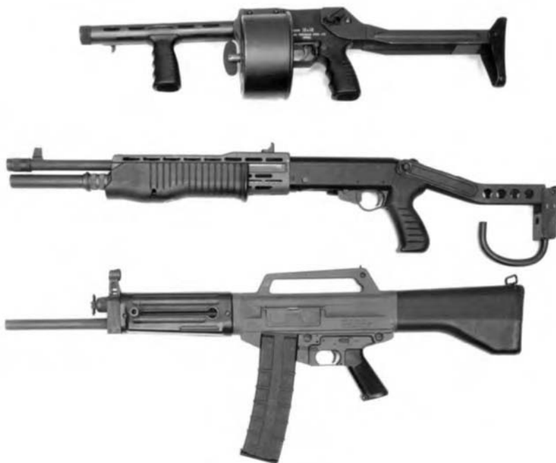
Figure 2.3 Shotguns of the type prohibited under the Firearms (Amendment Act) 1988. The Israeli “Dragon” 12-shot revolver gun, the Italian Franchi “SPAS 12” eight-shot pump-action/self-loader, and the Korean manufactured “USAS 12” self-loading gun available with detachable 10-shot box or 20-shot drum magazine (also available in full-automatic capability). All guns depicted are chambered for 12 bore ammunition.
