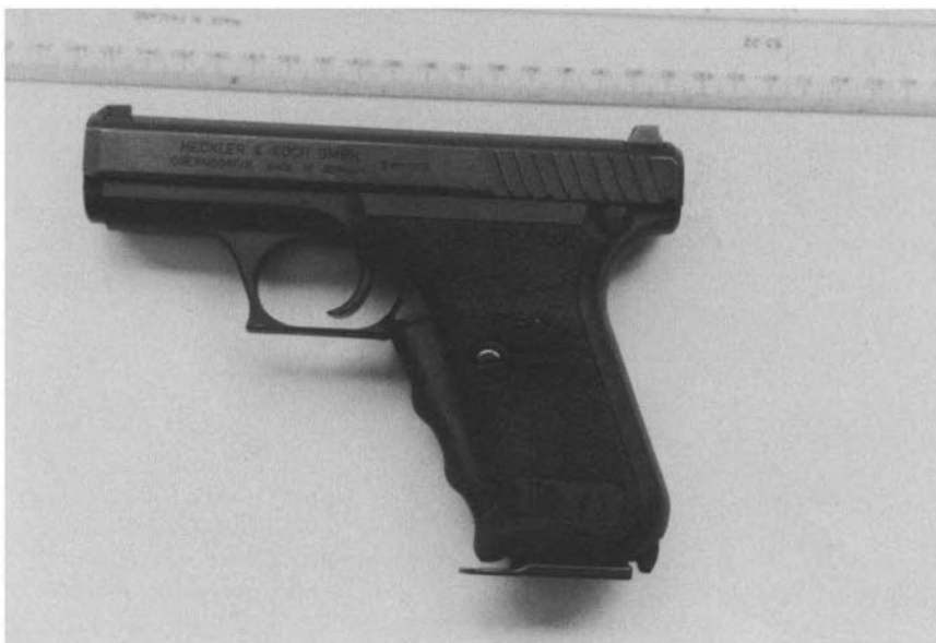
Figure 4.7 Heckler and Koch innovative gas retarded P7 9 mm self-loading pistol which utilises a squeeze-cocking/decocking device built into the grip.
