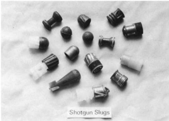
Figure 6.2 An assortment of shotgun slugs, which include Balle Blondeau diabolo shaped missiles, rifled and unrifled hollow Foster slugs, the ever-popular Brenneke slug, the Sellier and Bellot S-Ball, spherical and lethal ball and a barricade penetrating Ferret CS bomblet.
