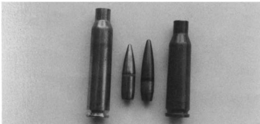
Figure 6.17 5.56x45 Nato versus the Soviet 5.45x39 loading. The use of a slightly smaller calibre and a steel core bullet enhances the ballistic shape of the Soviet loading as well as conferring a significant improvement in its ability to defeat light screening cover. The relatively new Nato SS109 bullet configuration which has replaced the original plain lead core loading, includes a part steel core and an increased weight to achieve similar enhanced downrange performance and penetration.
