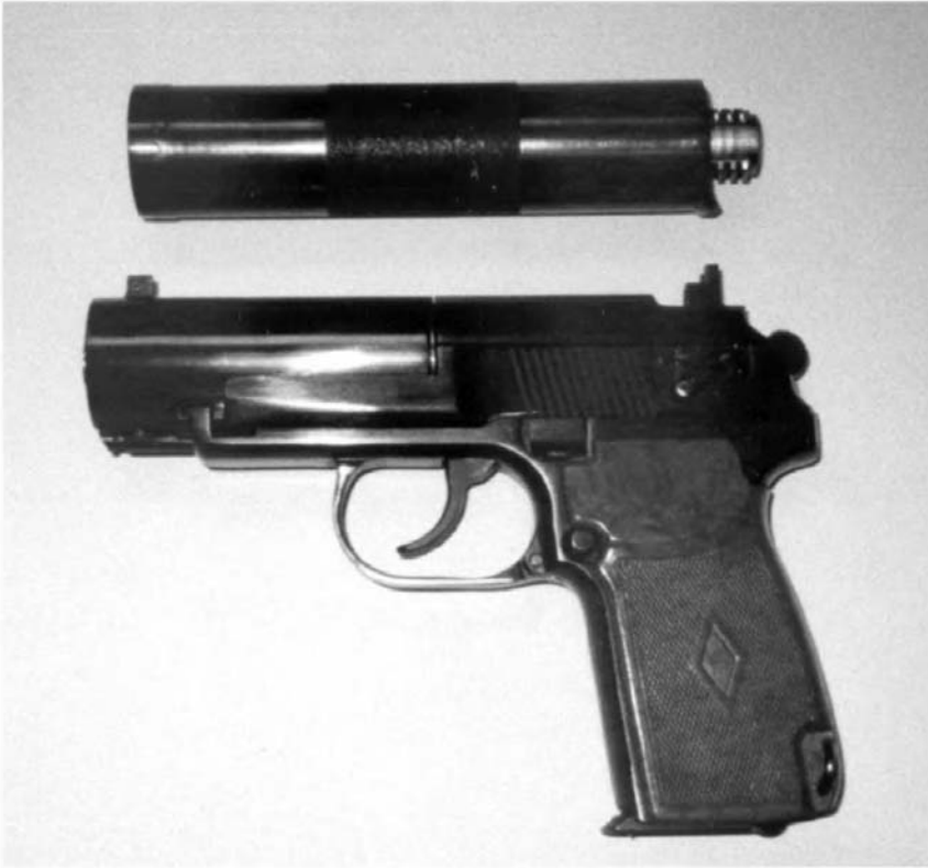
Figure 4.18 Russian special purpose 9 mm pistol with barrel assembled with integral silencer.
