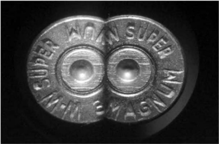
Figure 9.26 Another view of matching breech face impressions on cartridge cases.
