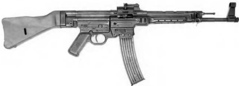
Figure 2.13 World War II German Sturmgeschütz Stg .44 assault rifle, chambered for the intermediate power 7.92 mm Kurz cartridge, gave Kalashnikov the inspiration during combat he experienced on the Eastern Front, to design the AK47 and AKM assault rifles, chambered for a cartridge of similar power, the M.43 7.62x 39 mm.
