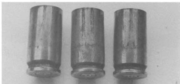
Figure 9.24 Distinctive chamber fluting marks left upon 9 mm cartridge cases fired in a weapon of Heckler and Koch manufacture. Such distinctive effects greatly support or shorten the computer search for weapon type.
