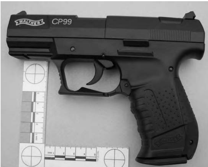
Figure 9.50 Walther CP99 carbon dioxide-powered repeating .177in/4.5 mm pistol.
