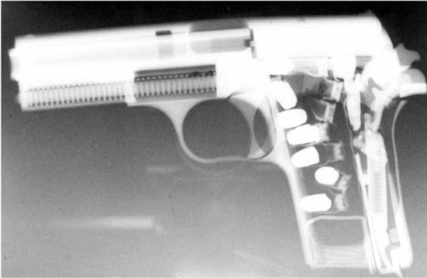
Figure 9.2 X-ray plate of seized-up fire damaged pistol reveals that the cartridges inside its magazine have been caused to explode by the heat. The picture confirms that it is now safe to attempt to free the pistol and attempt its dismantling.
