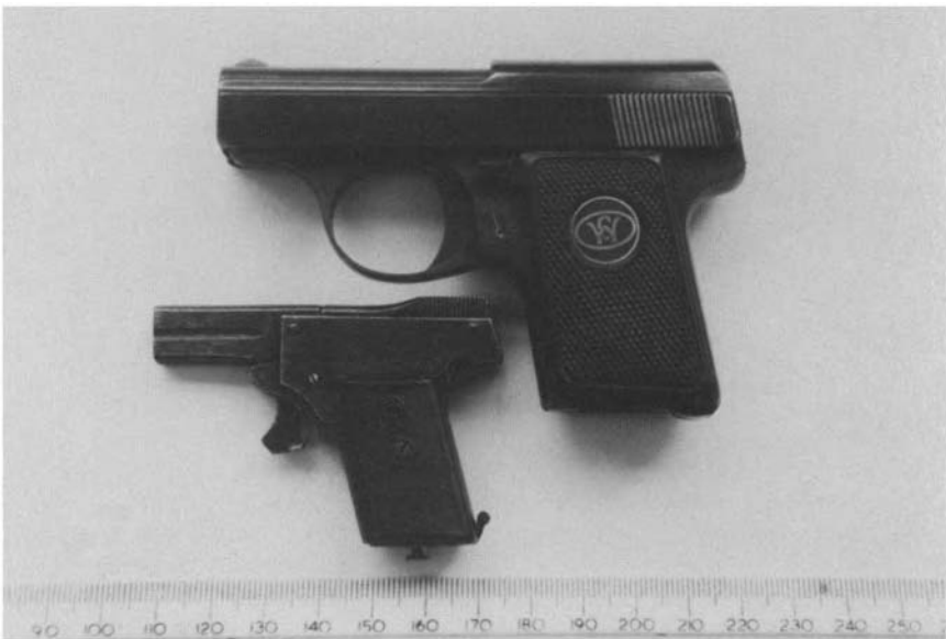
Figure 4.5 Even the tiny Walther Model 9 .25 in (6.35 mm) self-loading pistol looks huge next to the 2.7 mm Kolibri.
