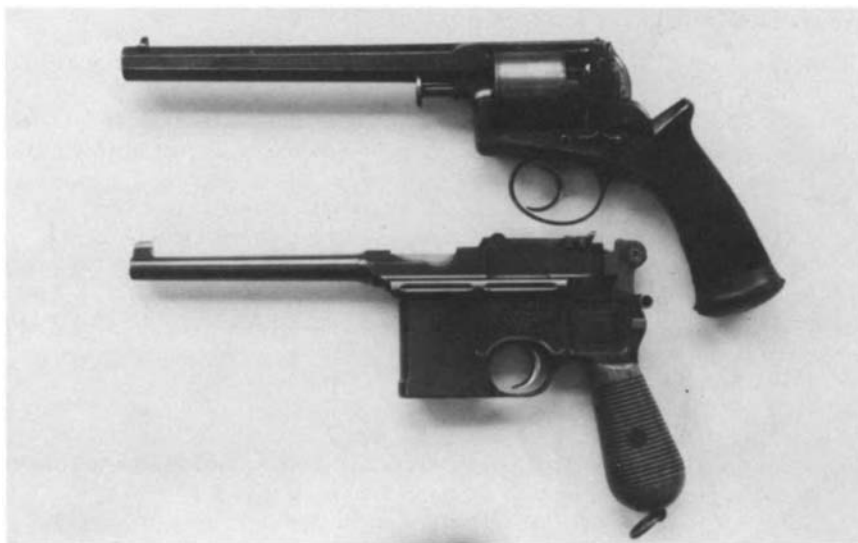
Figure 1.7 Powerful five-shot 38-bore (.50 in/12.7 mm) Adams double-action muzzle-loading percussion revolver of the mid-nineteenth century and the famous Mauser 10-shot self-loading recoil operated pistol of 1896 represent the dramatic pace of arms developments over the latter half of this century. The Mauser pistol loadings generated advertised muzzle velocities of 1410 ft/s (430 m/s).
