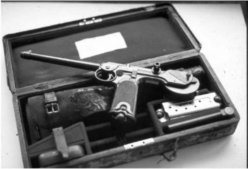
Figure 1.5 The Borchardt recoil-operated self-loading pistol of 1893 was chambered for a 7.65 mm cartridge employing a charge of nitrocellulose powder and a jacketed bullet. Shown here in its case with attachable shoulder stock.
