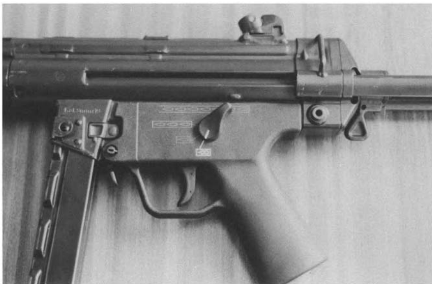
Figure 4.12 Heckler and Koch trigger grouping with fire selector to suit all tastes. Pictorial markings which minimise any language barrier indicate—safe, single-shot, three round burst or full—automatic modes of operation. Optional groupings calling up burst-fire operation involving a different number of cartridges are available.
