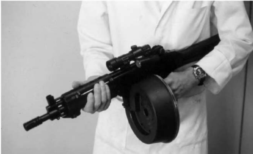
Figure 2.12 Post Firearms (Amendment) Act 1988 5.56 millimetre self-loading AR-18 design based carbine fitted with 90-round drum magazine, marketed as a “target pistol.” The screw used for providing additional security for attaching the shoulder stock to its body was not supplied, and the title “Pistol” was inscribed upon its side, in an attempt to circumvent the ban on self-loading centre-fire rifles and carbines.
