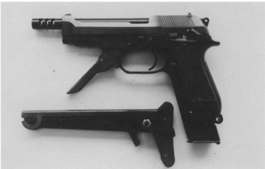
Figure 2.6 Burst-fire arms such as this Beretta Model 93R 9 mm pistol were also classified as prohibited weapons by the 1988 legislation. Weapon shown with attachable shoulder stock and 20-round magazine is designed to allow either one shot to be fired each time the trigger is pressed or a burst of three rounds at a very high cyclic rate.
