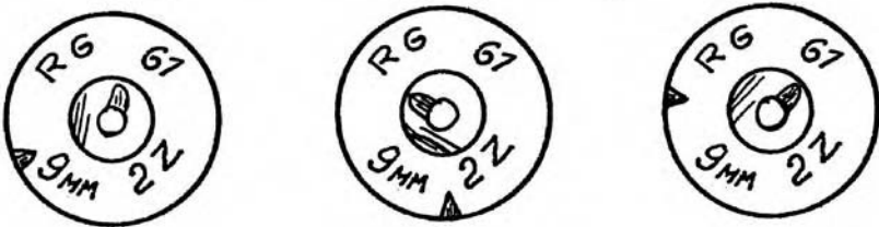
Figure 9.19 Fired cartridge cases showing the locations of operational markings.
