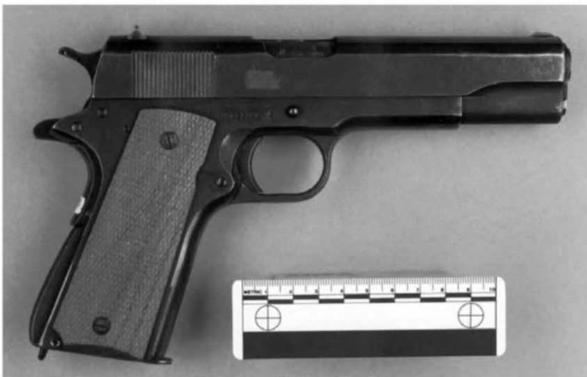
Figure 2.9 Zinc alloy imitation firearm resembling Colt .45 inch Model 1911-A1 self-loading pistol.
