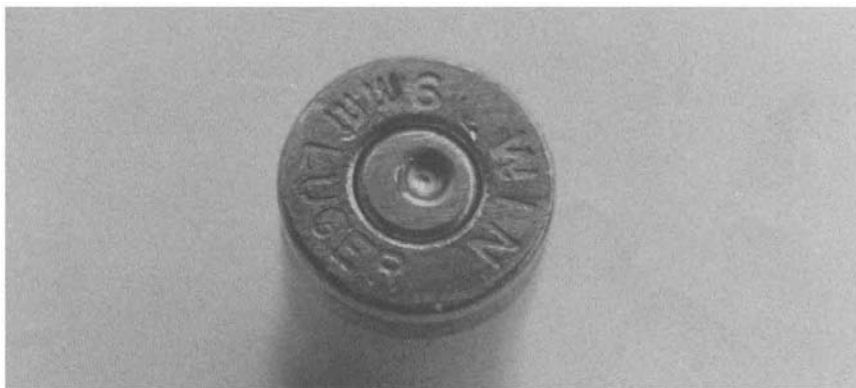
Figure 9.22 The unusual location of the ejector impact mark at 2 o'clock near to the primer is characteristic in this instance of the use of a Polish Radom P35 9 mm self-loading pistol.
