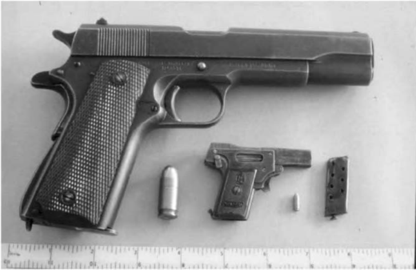
Figure 4.4 Diminutive but potentially lethal Kolibri 2.7 mm self-loading pistol of 1914 next to Colt Model 1911A1 .45 in pistol. Claimed ballistics for the Kolibri loading was a 3 grain (0.2 g) bullet at 650–700 ft/s (198–213 m/s) for a striking energy of 3 ft lb (4 J).
