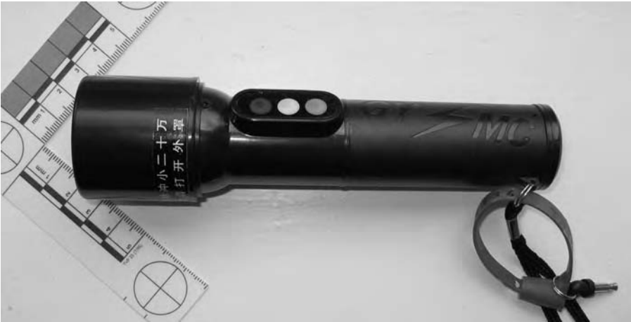
Figure 9.48 Stun gun disguised as a working flashlight.
