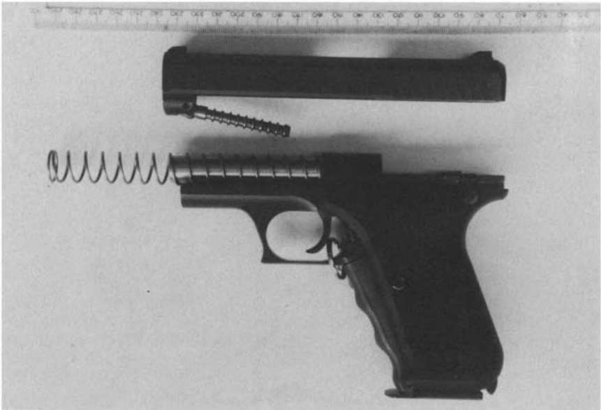
Figure 4.8 P7 pistol partially dismantled to reveal gas piston arrangement attached to front end of the slide.
